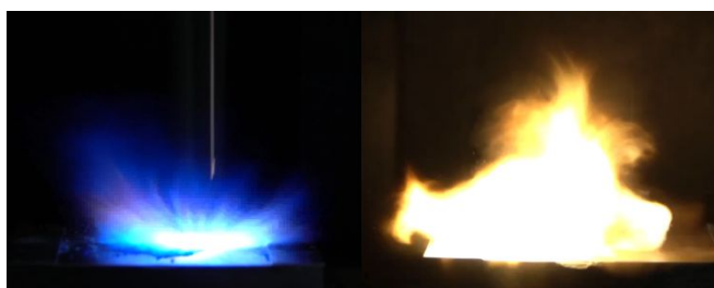
Figure 13. Moment of detonation during ball drop impact sensitivity measurements of the copper(II) perchlorate ( 13 ) and copper(II) azide complexes ( 14 )
