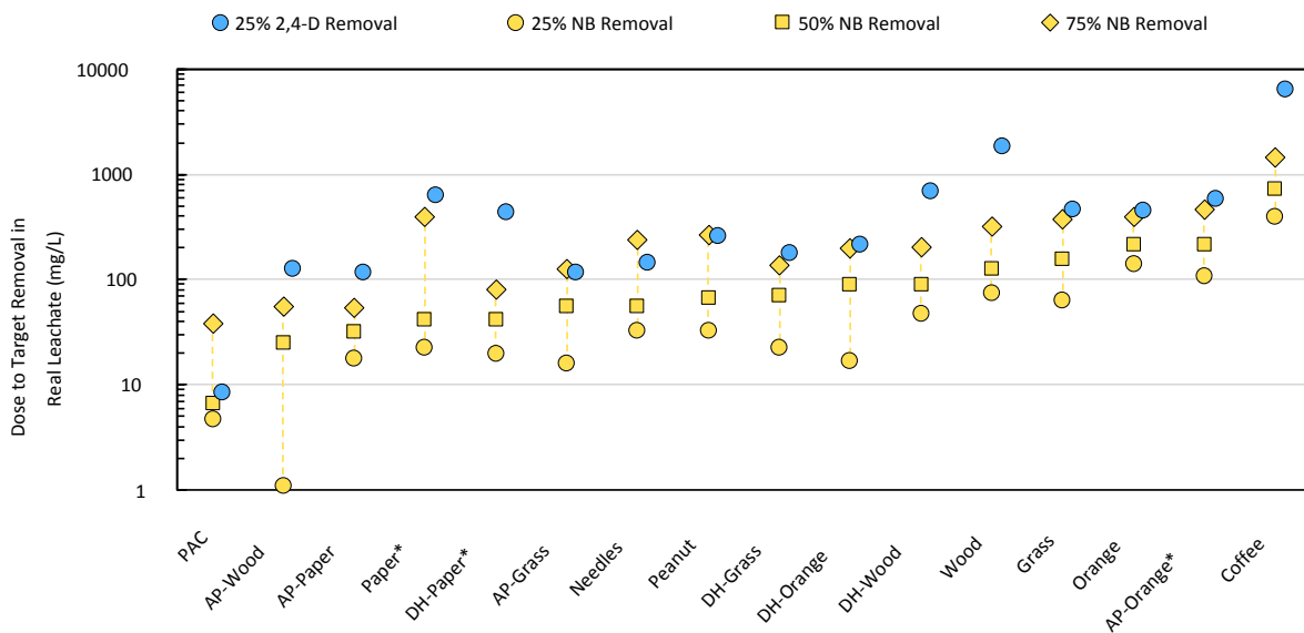
Figure 1. Representation of the dose response curves for the removal of 2,4-D (blue) and nitrobenzene (NB) (yellow) in real leachate for each adsorbent, including the ash-pretreated (AP) and double-heated (DH) biochars. Dose response curve values include 25% (circles), 50% (squares), and 75% (diamonds) removals. Note: * denotes extrapolated values for 25% 2,4-D removal.
