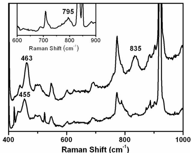
**Figure 5.** Resonance Raman spectra of **2A** in MeCN collected at 77 K with 413.1-nm excitation (100-mW power). Top:  $^{16}\text{O}$ -labeled **2A**; bottom:  $^{18}\text{O}$ -labeled **2A**. Inset:  $^{18}\text{O}$ -labeled **2A** spectrum obtained in  $\text{CD}_3\text{CN}$  to unmask the downshifted  $^{18}\text{O}$  vibration.
