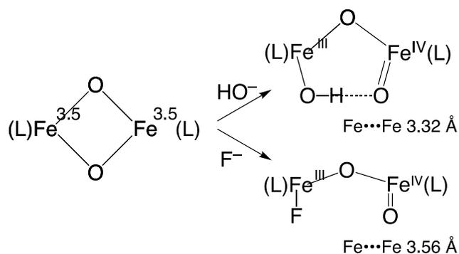
**Scheme 4:** Conversion of the valence-delocalized diamond core of **3A** into a valence-localized open X–Fe<sup>III</sup>–O–Fe<sup>IV</sup>=O core upon binding of OH<sup>−</sup> or F<sup>−</sup> to the Fe<sup>III</sup> site to generate a more highly reactive terminal S = 2 Fe<sup>IV</sup>=O unit.<sup>9b,9c</sup>
