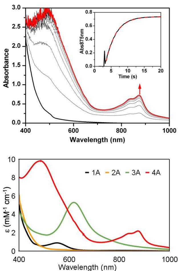
**Figure 2:** A (top): Formation of **4A** from the reaction of 0.3 mM **2A** in MeCN with 1 equiv. 70% H<sub>2</sub>O<sub>2</sub> at -40°C in 85% yield as determined by UV-Vis spectroscopy. B (bottom): Comparison of electronic spectra of **1A**, **2A**, **3A**, and **4A**, showing the significantly more intense visible/near IR features of the higher-valent complexes.
