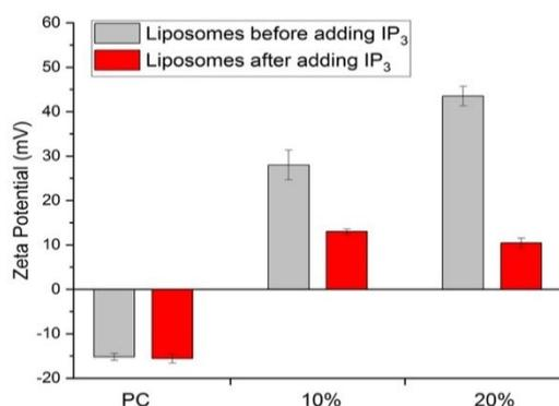
**Figure 2.** Zeta potential measurements for 0, 10, or 20% **1**/PC liposomes before and after adding IP<sub>3</sub>. Both 10% and 20% liposomes exhibited positive charge initially, while IP<sub>3</sub> addition yielded a reduction in positive charge. PC liposomes showed virtually no ZP changes after IP<sub>3</sub>. Error bars denote standard errors from three replicates.
