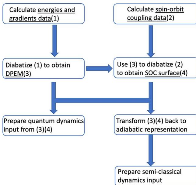
Figure 1. Diagram for constructing a DPEM including SOC data and using the DPEM for input to dynamics simulations
