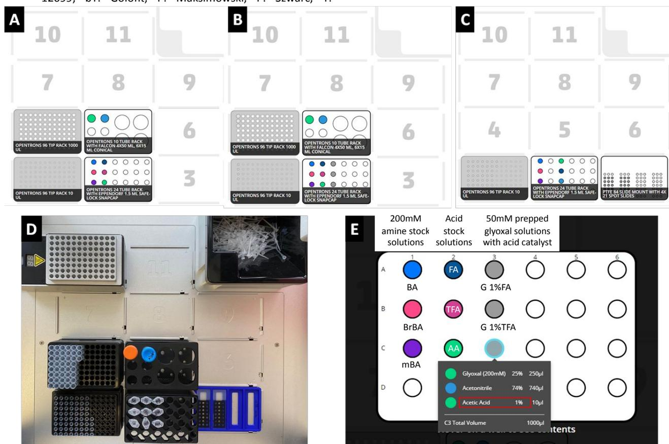
**Figure 1.** (A) Starting deck state of the Opentrons robot for the “DESI\_Prep” protocol (B) Final deck state of the Opentrons robot for the “DESI\_Prep” protocol (C) Final deck state of the Opentrons robot for the “DESI\_Spot” protocol (D) Picture of the deck layout (E) Zoomed view of Opentrons 24 Tube Rack from slot 2 in final deck state of “DESI\_Prep” protocol.
