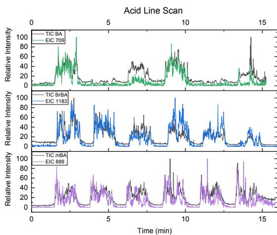
**Figure 4.** Total ion chromatogram (TIC) and extracted ion chromatograms (EIC) are shown for the acid screening DESI slide. The line scan includes six spots with formic acid spotted in the 1st and 4th position, trifluoroacetic acid spotted in the 2nd and 5th position, and acetic acid spotted in the 3rd and 6th position. The EIC for benzylamine product ( $m/z$  709) is in green, blue for the bromo-benzylamine product ( $m/z$  1183), and the methoxy benzylamine ( $m/z$  889) in purple.
