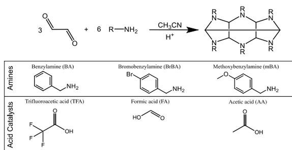
**Scheme 1.** Condensation reaction step to form HBIW intermediate. Traditional HBIW formation is carried out with benzylamine and formic acid. Bromo- and methoxybenzylamine were substituted in this reaction to form HBIW analogs. Formic acid was also substituted with trifluoroacetic acid and acetic acid to screen acid catalysts.
