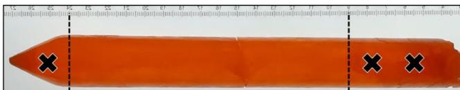
Figure 2. A typical zone refined crystal showing the region that is discarded before using it as charge material for a VB growth.
