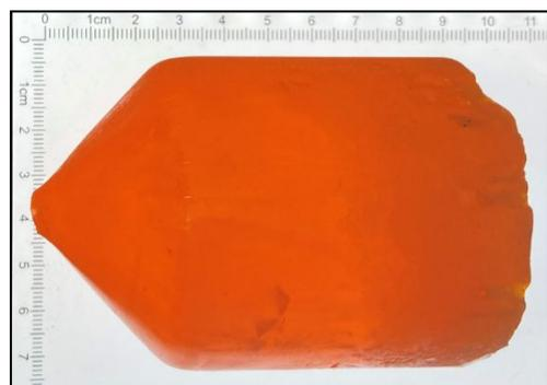
Figure 4. 65 mm diameter CsPbBr<sub>3</sub> single crystal, largest ever produced. The inhomogeneities in the crystal color are limited only to the surface.
