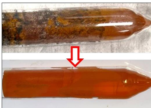
Figure 3. As-grown CsPbBr<sub>3</sub> crystals before and after optimization of the purification process.
