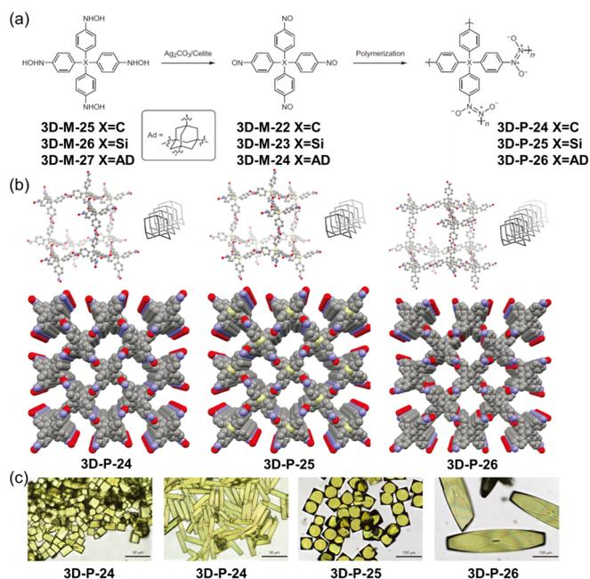
**Fig. 35** Diamondoid azidoxy 3D SCFs: (a) Synthesis of three covalent organic networks **3D-P-24**, **3D-P-25**, and **3D-P-26** by reversible self-addition polymerizations; (b) Single-crystal structures of **3D-P-24**, **3D-P-25**, and **3D-P-26**; (c) Optical microscopy images of the single crystals **3D-P-24**, **3D-P-25**, and **3D-P-26**. Reproduced with permission from ref. 10, Copyright 2013, Springer Nature.
