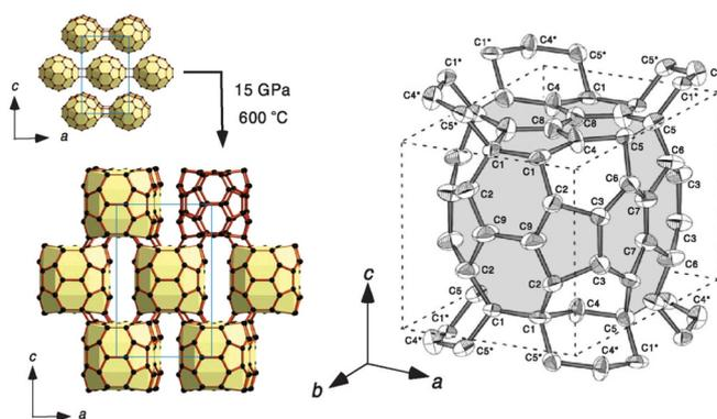
**Fig. 36** Single-crystal structure of the 3D C<sub>60</sub> SPC **3D-P-27**. Reproduced with permission from ref. 208, Copyright 2023, American Physical Society.
