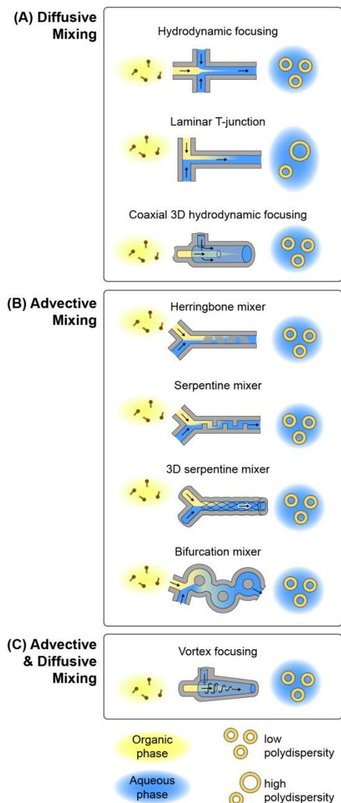
**Fig. 3: Microfluidic lipid nanoparticle production technologies.**
