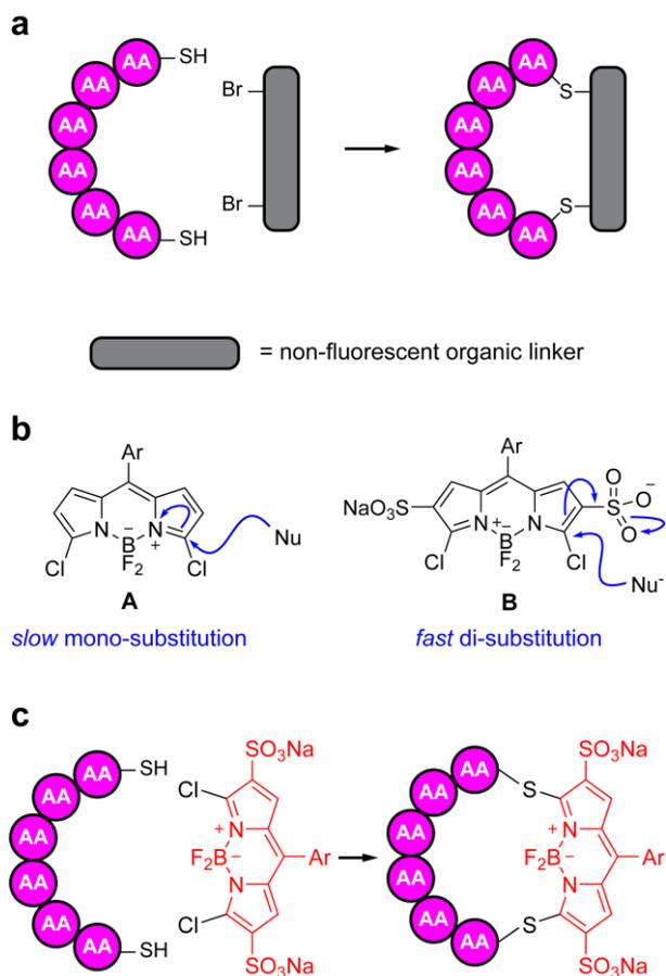
**Fig. 1.** **a** Typical CLIPS or CLIPS-like construction of cyclic peptides where S-containing residues selectively displace a benzylic or aromatic halide. **b** Non-sulfonated BODIPY **A** undergoes  $S_NAr$  slower and requires harsher conditions less suitable to peptide chemistry than the disulfonated BODIPY **B**. **c** The intrinsically fluorescent *cyclo*-organopeptides synthesized and explored in this paper.
