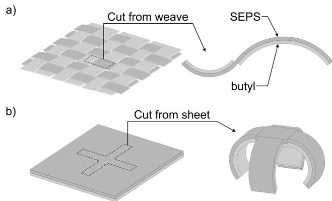
Fig. 3 Schematics showing a cut out from a) an interwoven mesh of butyl and SEPS that forms the two-segment alternating bilayer strip and b) a bilayer sheet that forms the bilayer cross, curling into a grasper following tensioning and release. Butyl is shown in light grey and SEPS is shown in darker grey.
