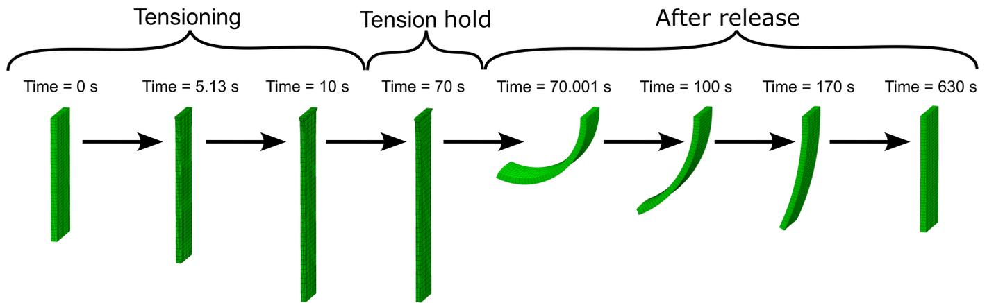
Fig. 4 FEA bilayer strip simulation overview. The PRF Power Law 20 mm 2 mm/s 60 s simulation is shown.
