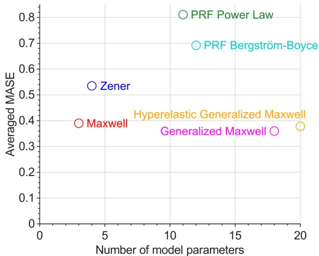
Fig. 9 Averaged MASE across all tests vs number of model parameters. Averaged MASE values per test are shown in supporting information Table S1.
