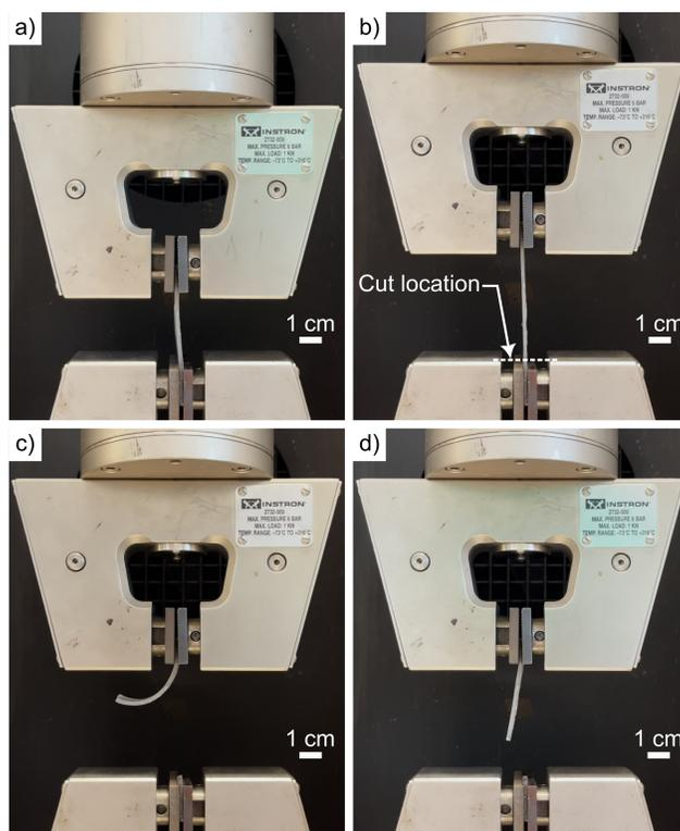
Fig. 1 Bilayer curvature testing procedure shown on a 20 mm extension test at a  $2 \text{ mm/s}$  extension rate with a hold time of 20 s. a) The bilayer sample is pre-tensioned until taut before undergoing a constant rate extension. b) The beginning of the bilayer sample's hold time following completion of extension. c) The sample shown 1.20 seconds after cutting. d) The sample after 10 minutes of relaxation.
