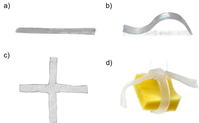
Fig. 10 Photographs of the two-segment alternating bilayer strip and bilayer cross. The two-segment alternative bilayer shown a) fully relaxed and b) shortly following tensioning and release. The bilayer cross shown c) fully relaxed and d) grasping a foam piece following tensioning and release (Supporting Movie S1).
