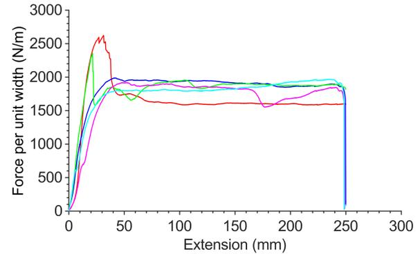
Fig. 6 SEPS-butyl adhesive testing results. Each coloured line corresponds to a different sample trial adhesive test.
