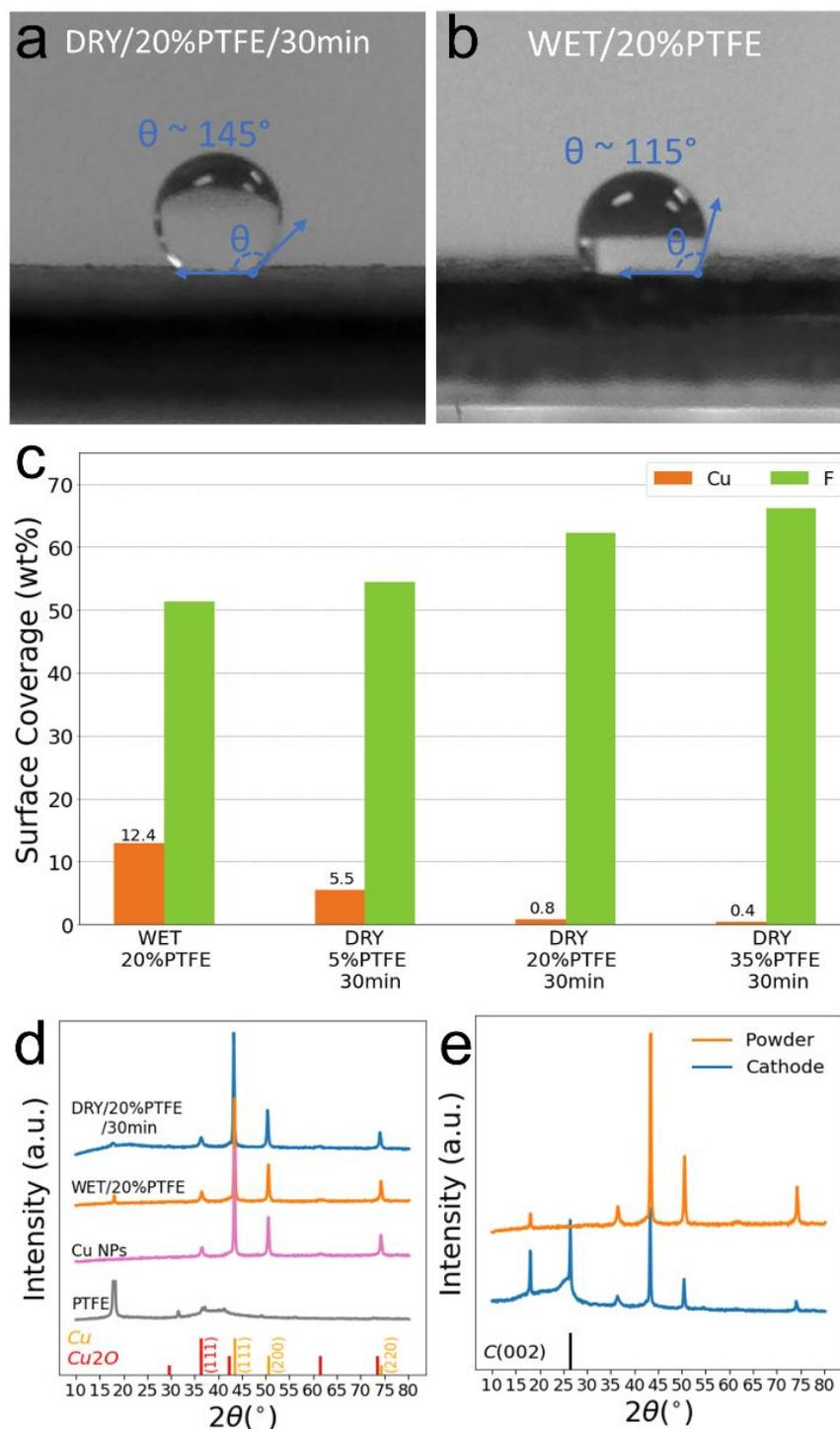
**Fig. 3.** Water contact angle measured on the cathode made of (a) DRY/20%PTFE/30min and (b) WET/20%PTFE; (c) Surface elemental composition of Cu and F on various catalysts as determined by XPS; (d) XRD patterns of precursor materials, DRY/20%PTFE/30min, and WET/20%PTFE; (e) XRD patterns comparing DRY/20%PTFE/30min catalyst and the resultant cathode.
