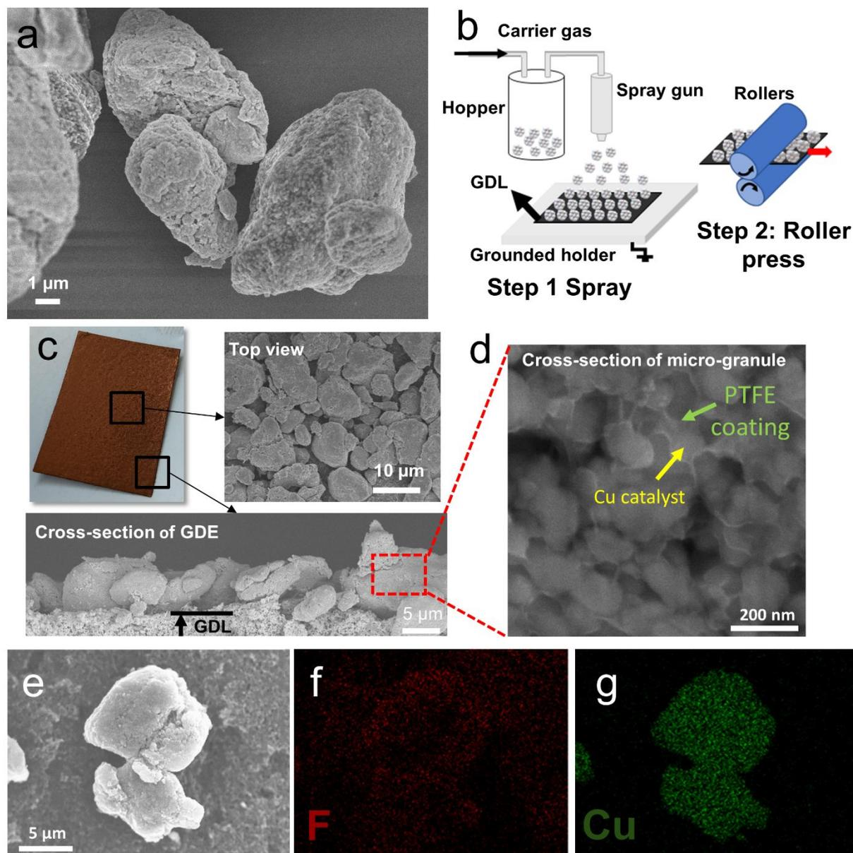
**Fig. 2.** (a) SEM image of prepared micro-granules. (b) Graphical representation of the electrostatic spray and roller press to fabricate the GDE. (c) A typical completed cathode with SEM images from a top view and a cross section view. (d) FIB-SEM cross-section image of a micro-granule. (e, f, g) EDS elemental mappings of the micro-granule deposited onto a GDL via EDS.
