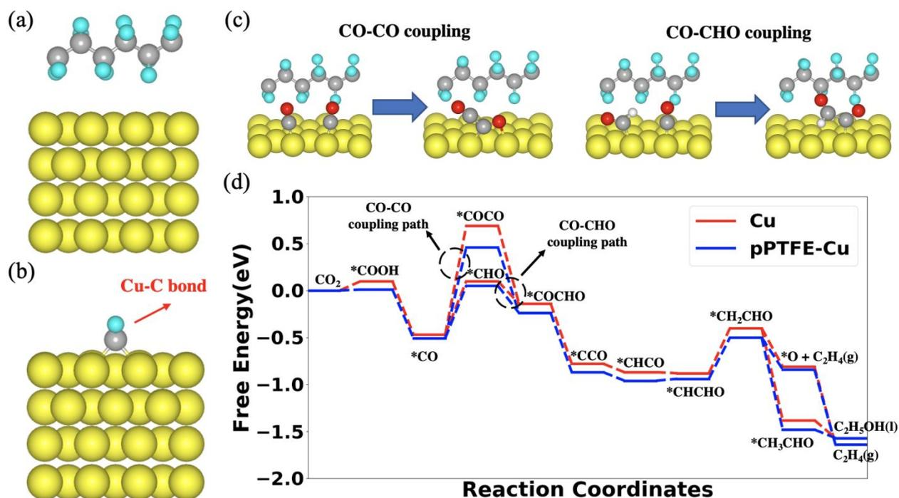
**Fig. 6.** Atomistic structures of (a) physical adsorption configuration of PTFE on Cu(111), (b) chemical adsorption configuration of PTFE on Cu(111), and (c) the CO-CO and CO-CHO coupling process. Here, the yellow, grey, cyan, red, and white balls represent Cu, C, F, O, and H atoms, respectively. (d) Predicted free energy evolution for CO<sub>2</sub> reduction to C<sub>2</sub> products on clean Cu(111) and pPTEF-Cu(111) surfaces.
