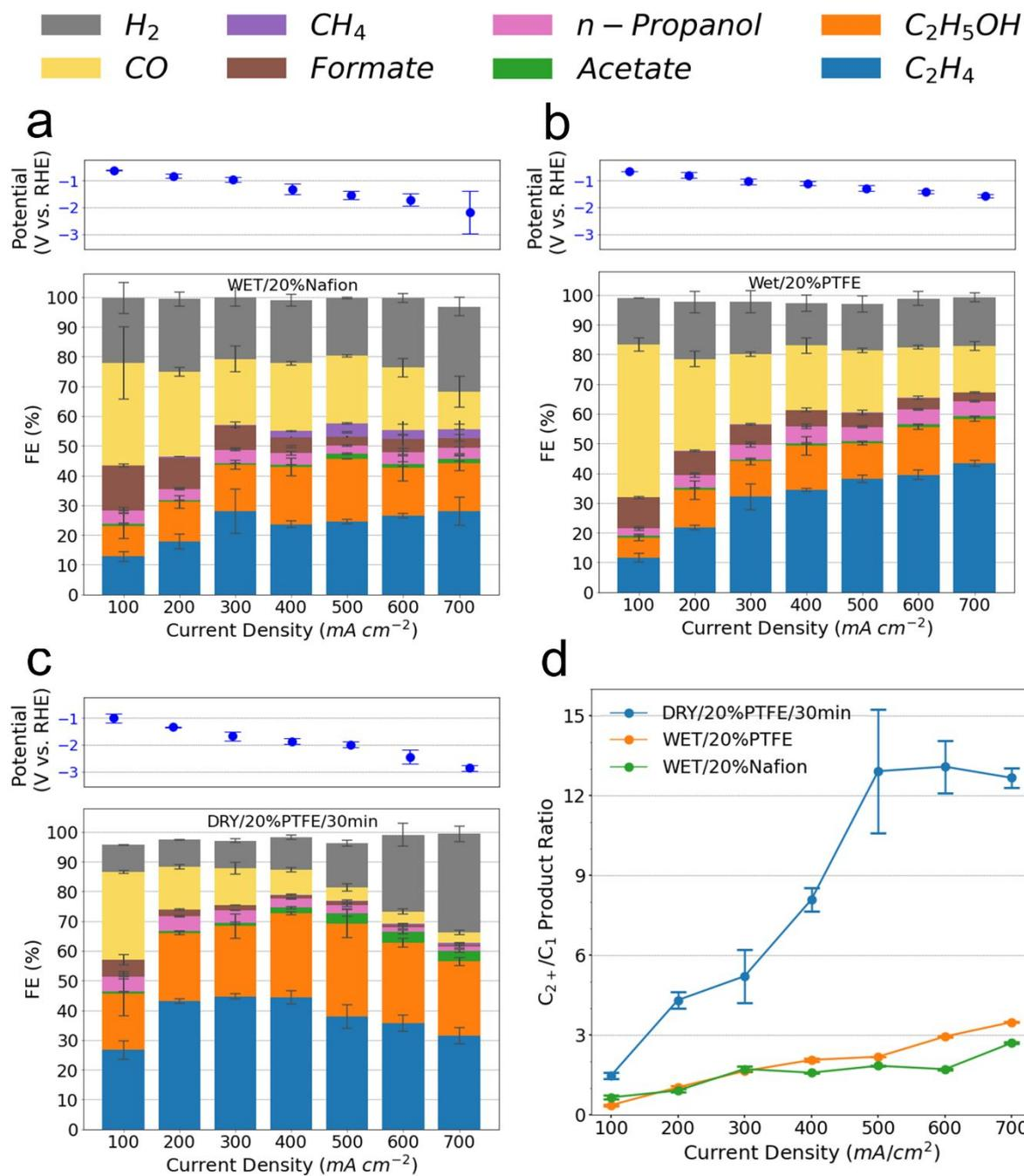
**Fig. 5.** Comparison of electrochemical performances of DRY and WET samples (a) WET/20%Nafion, (b) WET/20%PTFE, (c) DRY/20%PTFE/30min regarding Faradaic efficiency and working potential over a range of applied current densities, and (d) comparison of  $C_2^+/C_1$  product ratios between DRY/20%PTFE/30min, WET/20%PTFE, and WET/20%Nafion over a range of applied current densities.
