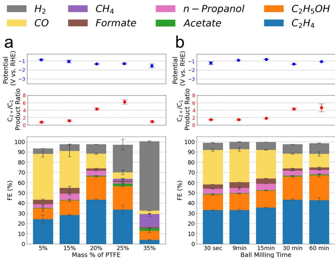
**Fig. 4.** Effects of a) PTFE mass loading and b) ball milling time in catalyst preparation on CO<sub>2</sub>RR product Faradaic efficiencies, C<sub>2+</sub>/C<sub>1</sub> product ratio, and working potential, tested in a flow cell at 200 mA cm<sup>-2</sup>.
