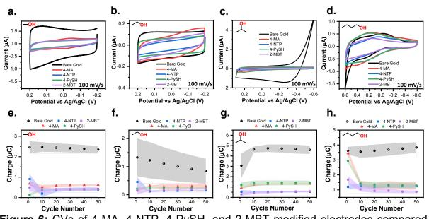
**Figure 6:** CVs of 4-MA, 4-NTP, 4-PySH, and 2-MBT modified electrodes compared to baseline CVs cycled within the SPWs established for 0.1 M LiCl (a) MeOH, (b) EtOH, (c) IPA, and (d) BuOH. The average integrated charge from the anodic sweeps of the baseline and modified electrodes CVs plotted versus the cycle number in (e) MeOH, (f) EtOH, (g) IPA, and (h) BuOH. The shaded regions depict the standard deviation of each measurement for three independent measurements.
