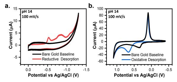
**Figure 1:** CVs in degassed 1 M KOH showing the **(a)** reductive desorption and **(b)** oxidative desorption of 4-PySH compared to baseline bare gold CVs.
