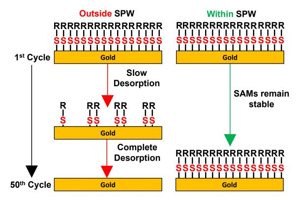
**Scheme 2:** Depiction of slow desorption of thiolate SAMs on gold in non-aqueous solvents when cycling to potentials outside the SPW and the retention of the SAM when cycled within the SPW.
