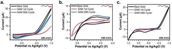
**Figure 5**: Comparing a baseline CV in 0.1M LiCl BuOH against a 4-MA covered electrode when **(a)** cycled negatively beyond the SPW and **(b)** when cycled positively beyond SPW. **(c)** A scheme of the SPW of thiolate SAMs in non-aqueous solvents.
