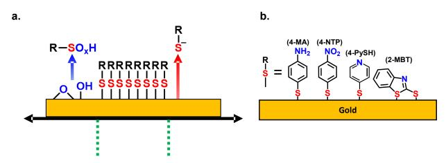
**Scheme 1: (a)** Depiction of the stable potential window (SPW) of thiolate SAMs on gold in aqueous solvents. **(b)** The thiol molecules used to investigate the SPWs: 4-mercaptoaniline (4-MA), 4-nitrothiolphenol (4-NTP), 4-mercaptopyridine (4-PySH), and 2-mercaptobenzothiazole (2-MBT).
