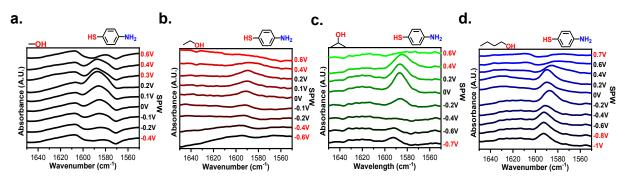
**Figure 7:** Spectra of a 4-MA modified SEIRAS substrate at different applied potentials within 0.1 M LiCl (a) MeOH, (b) EtOH (c) IPA, and (d) BuOH. The voltages marked in red denote applied potentials beyond the CV-based SPW.
