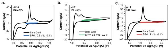
**Figure 2:** CVs of a bare gold electrode compared to a 4-PySH-covered electrode cycled within the SPW in **(a)** 1 M KOH (pH 14), **(b)** 0.1 M NaCl (pH 7), and **(c)** 0.1 M HClO<sub>4</sub> (pH 1).
