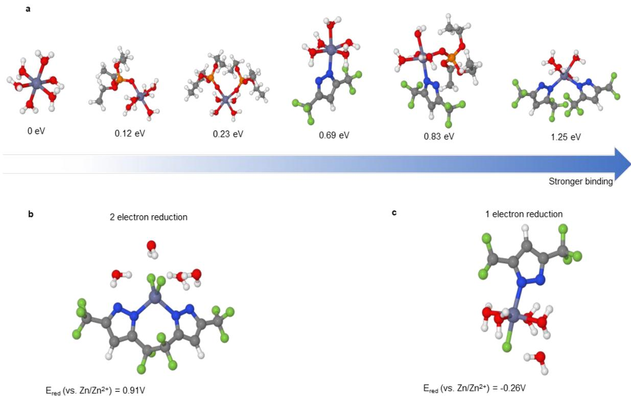
**Fig. 3: Proposed SEI formation mechanisms for TFMP.** **a**, Binding free energies from DFT calculations relative to  $\text{Zn}(\text{H}_2\text{O})_6$  in eV for various solvates comprising Zn,  $\text{H}_2\text{O}$ , TEP, and  $\text{TFMP}_{\text{H}}$ ; the latter of which is an anion in these solvates. Higher values mean stronger binding. **b-c**, DFT computed double (**d**) and single (**e**) electron reduction potentials of Zn solvates with two or one  $\text{TFMP}_{\text{H}}$  anions.
