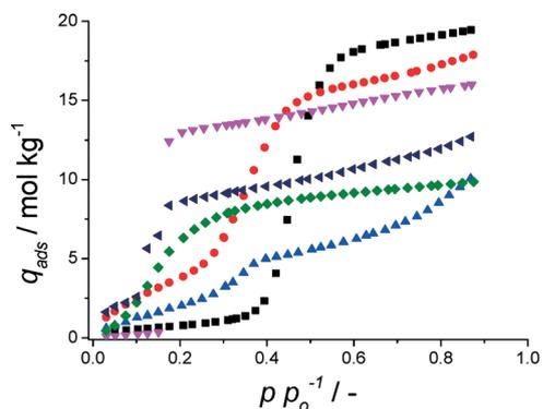
Fig. 1 H<sub>2</sub>O adsorption isotherms at 298 K of CAU-1 (■), CAU-1-(OH)<sub>2</sub> (●), CAU-8 (▲), CAU-10-H (▼), CAU-10-NH<sub>2</sub> (◆) and CAU-10-OH (◄).
