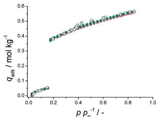
Fig. 4 Repeated  $\text{H}_2\text{O}$  adsorption isotherms at 298 K of CAU-10-H supported on a metallic aluminium plate. First ( $\blacksquare$ ), second ( $\bullet$ ), third ( $\blacktriangle$ ), fourth ( $\blacktriangledown$ ) and fifth ( $\blacklozenge$ ) measurements. Closed symbols depict adsorption, open symbols, desorption. Loading is presented as per total mass of sample (Al substrate + CAU-10-H).
