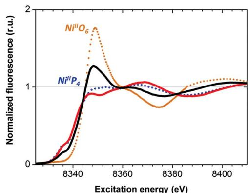
Fig. 4 X-ray absorption near edge structure spectra (Ni K edge) of the Ni-CNT material as prepared (black solid line), and after 1 h  $H_2$  oxidation (red solid line). Spectra of pristine  $[Ni(P^{Ph}N_2^{CH_2pyrene})_2]$  (blue dotted line) and of  $[Ni(OH_2)_6]^{2+}$  (orange dotted line) are shown for comparison. See Fig. S10† for a magnification of the K edge region.
