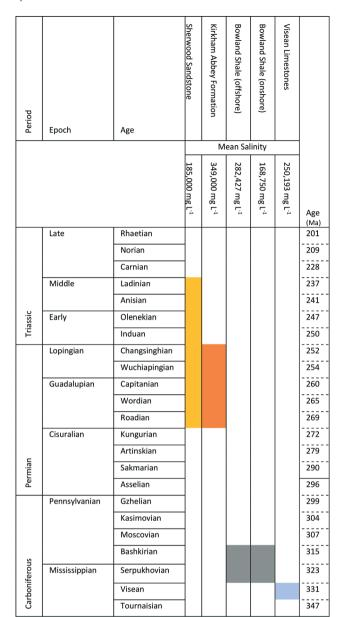
Fig. 2 Stratigraphic chart annotated with mean salinities (mg L<sup>-1</sup>) of FP and produced water data by source formation for the UK.
