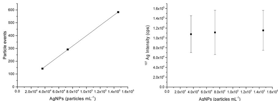
Fig. 1 External calibration with AgNPs. (Left) Measured number of AgNP events versus AgNP concentrations (equation: number of AgNP events =  $0.0040 \times [\text{AgNPs mL}^{-1}] - 2.90$ ;  $R^2 = 0.999$ ). (Right) Measured  $^{107}\text{Ag}$  in counts per second (cps) versus AgNP concentrations.
