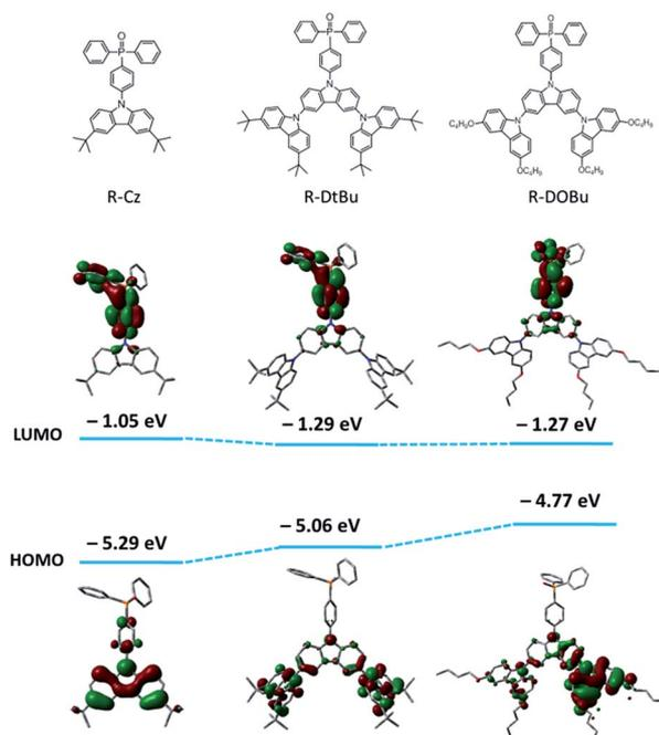
Fig. 2 Calculated HOMO/LUMO levels for the building blocks of the polymer hosts (B3LYP/6-31G(d)). The calculated HOMO level shifts from  $-5.29$  eV to  $-5.06$  eV and  $-4.77$  eV in the order of R-Cz, R-DtBu and R-DOBu, consistent with the experimental results ( $-5.64$ ,  $-5.37$  eV and  $-5.20$  eV for PH3, PH1 and PH2, respectively).
