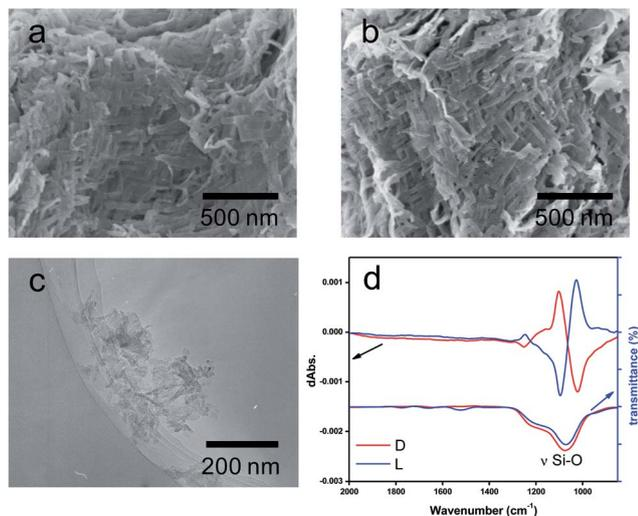
Fig. 1 SEM images of calcined silicas, (a)  $D$ - $SiO_2$ -600 and (b)  $L$ - $SiO_2$ -600. TEM images of (c) the piece of  $L$ - $SiO_2$  crushed by homogenizing the methanol solution containing chiral silica bundles (calcined PEI/tart@ $SiO_2$ ) for at least 20 000 rpm for 2 min. (d) FT-IR/VCD spectra of the crushed  $SiO_2$ , red lines for the  $D$ -form, and blue lines for the  $L$ -form.
