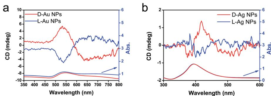
Fig. 6 CD and UV-vis spectra of (a) chiral Au NPs and (b) Ag NPs dispersed in water obtained from the hydrolysis (by using 5 wt% NaOH) of chiral Au@SiO<sub>2</sub>-500 and Ag@SiO<sub>2</sub>-600, respectively.
