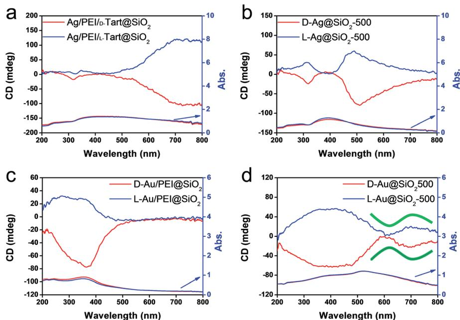
Fig. 3 DRCD and UV-vis spectra of (a) Ag/PEI/tart@SiO<sub>2</sub>, (b) Ag@SiO<sub>2</sub>-500, (c) Au/PEI@SiO<sub>2</sub> and (d) Au@SiO<sub>2</sub>-500, red lines for D-form and blue lines for L-form.
