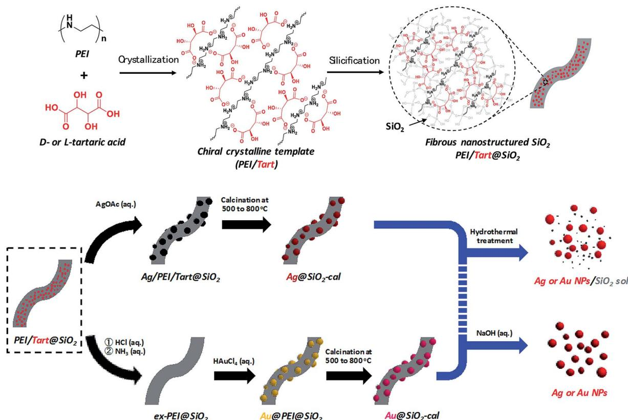
Scheme 1 Representation of the procedure for obtaining chiral SiO<sub>2</sub> and metal@SiO<sub>2</sub> composites and two approaches for isolation of metal NPs from the metal@SiO<sub>2</sub> composites.
