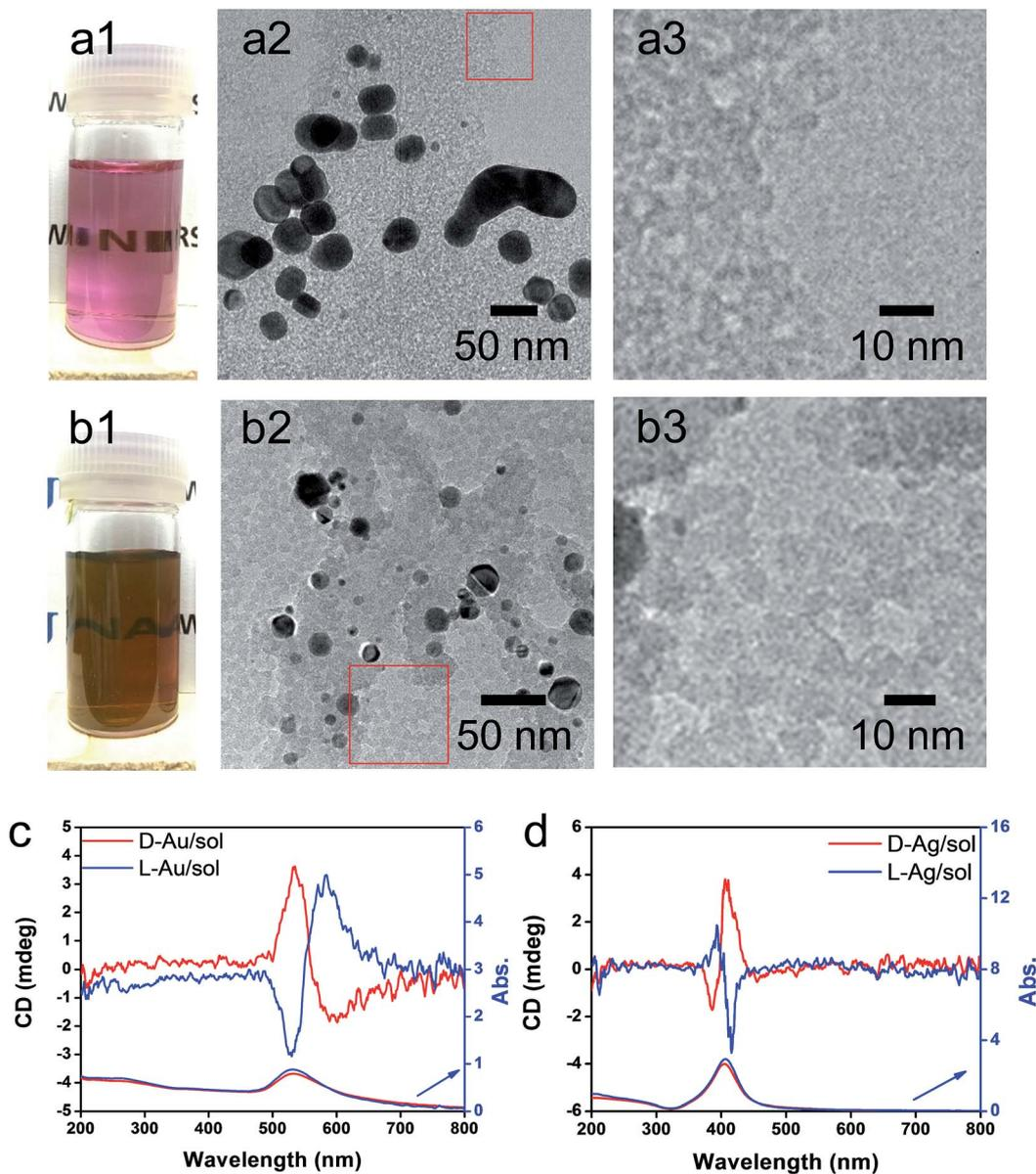
Fig. 4 Aqueous solution of L-Au/sol (a1) and L-Ag/sol (b1). TEM images at different magnifications of L-Au/sol (a2 and a3) and L-Ag/sol (b2 and b3) (taken from a highly diluted solution containing Au/sol or Ag/sol). CD and UV-vis spectra of Au/sol (c) and Ag/sol (d) (both samples were diluted from their stock solutions), red lines for the D-form and blue lines for the L-form.
