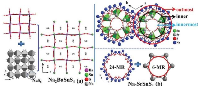
Fig. 2 (a) Crystal structure of  $\text{Na}_2\text{BaSnS}_4$  along the *c*-axis: a 3D network composed of edge-sharing  $\text{BaS}_8$  dodecahedra, and an edge and corner-sharing  $(\text{NaS}_6)_n$  3D network; (b) the whole structure of  $\text{Na}_2\text{SrSnS}_4$ : three-types of rings (outermost, inner, innermost), 24- $\text{NaS}_6$ -MR, and 6- $\text{SrS}_7$ -MR.
