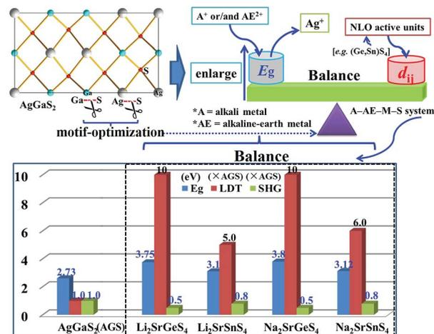
Fig. 6 Schematic diagram of designing new IR NLO materials by the motif-optimization with  $\text{AgGaS}_2$  as the template and title compounds achieve the suitable balance of wide  $E_g$  and good  $d_{ij}$ .
