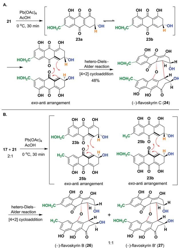
Scheme 3 (A) Oxidation of 21 by Pb(OAc)<sub>4</sub> forms (–)-flavoskyrin C (24) through the hetero Diels–Alder reaction. (B) Oxidation of a mixture of 17 and 21 (2 : 1) by Pb(OAc)<sub>4</sub> yielded flavoskyrin B (26) and flavoskyrin B' (27) as a major product.
