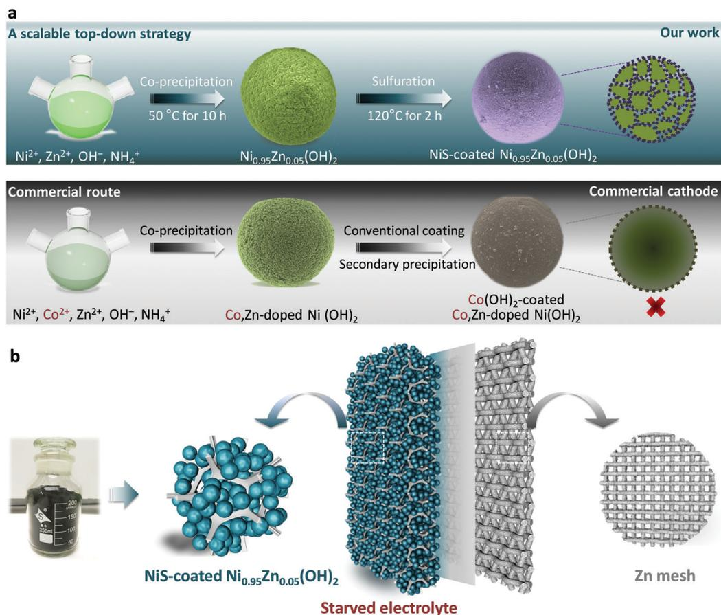
**Scheme 1** The scalable top-down strategy for application in Ni–Zn batteries. (a) Schematics showing the preparation steps of the top-down strategy compared with the existing commercial route. (b) Electrode configuration and specification of the Ni–Zn battery. The inset shows the industrial viability of the strategy.
