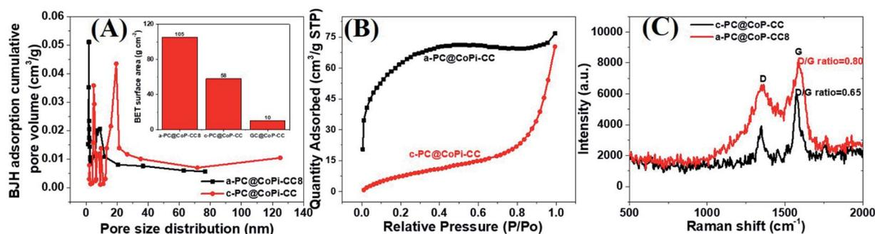
Fig. 4 BJH pore distribution (A), where the inset shows the BET surface area of the different samples. N<sub>2</sub> adsorption isotherms (B) and Raman spectra (C) of the a-PC@CoPi-CC8 and c-PC@CoPi-CC.
