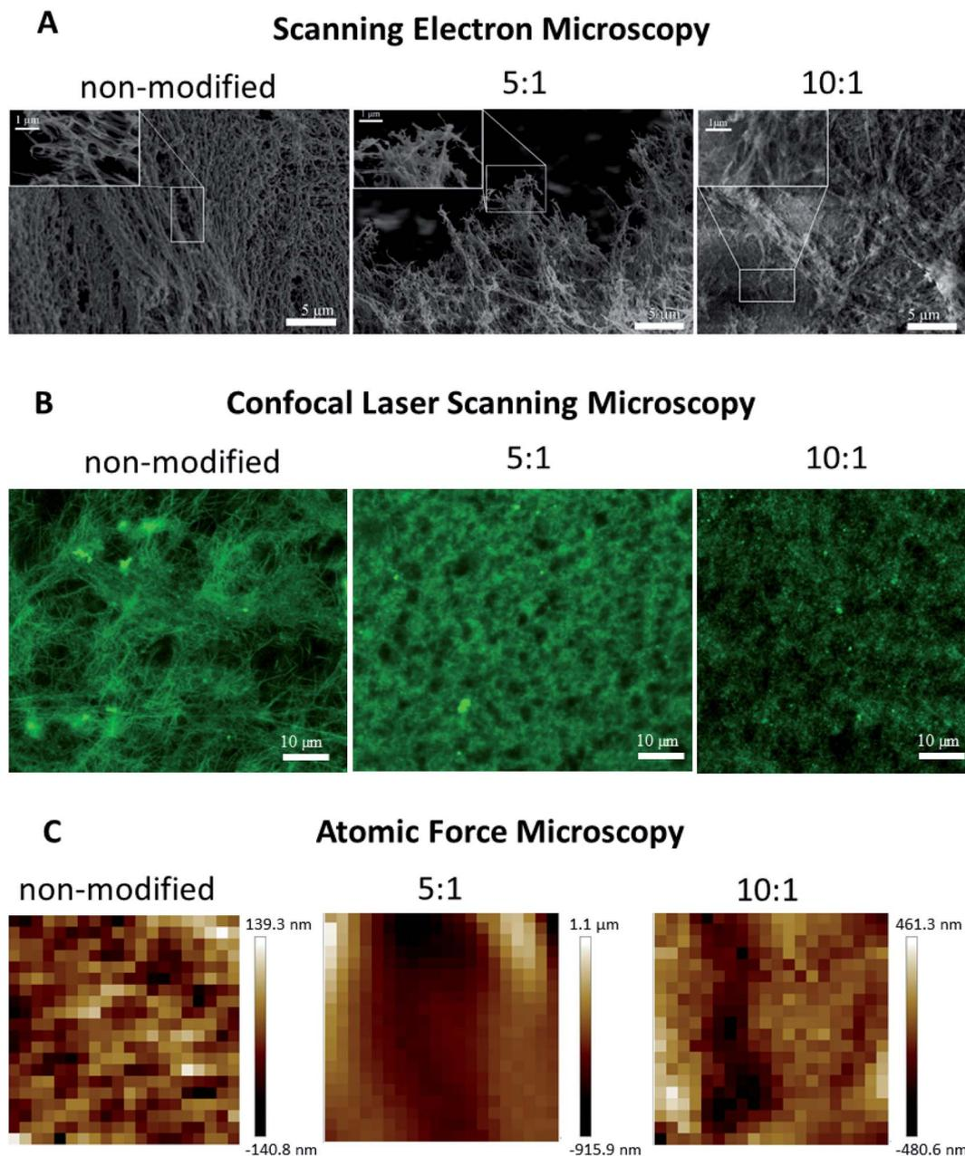
**Fig. 3** (A) SEM images of non-modified, 5 : 1 PEGylated, and 10 : 1 PEGylated fibrin gels. (B) Confocal laser scanning microscopy images of gels. The PEGylation degree determined the fiber morphology and packing: compared to the non-modified gel, 5 : 1 and 10 : 1 PEGylated fibrin had a flocculent structure. (C) Topography maps over a 30 × 30 μm area showing different scales of inhomogeneity in the gels.
