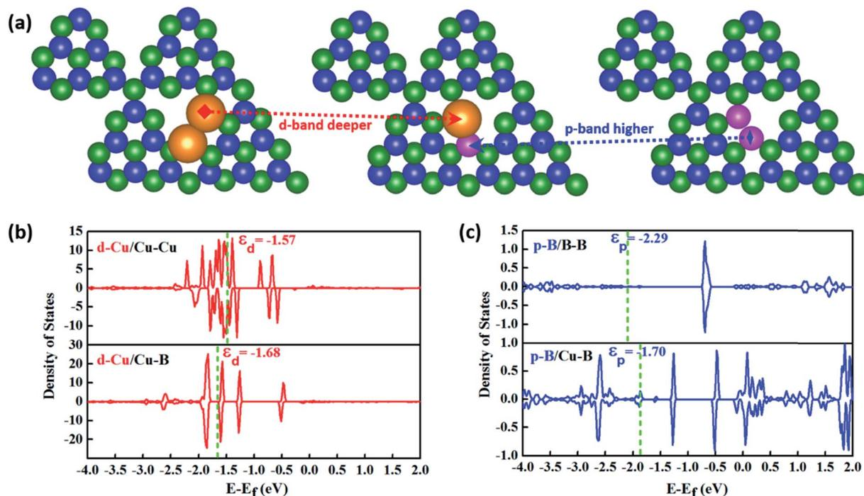
Fig. 4 (a) Structural models for Cu–Cu, Cu–B and B–B anchored on g-C<sub>3</sub>N<sub>4</sub>. The d-band centers of Cu in (b) Cu–Cu@g-C<sub>3</sub>N<sub>4</sub> and Cu–B@g-C<sub>3</sub>N<sub>4</sub>, and p-band centers of B in (c) B–B@g-C<sub>3</sub>N<sub>4</sub> and Cu–B@g-C<sub>3</sub>N<sub>4</sub>. Green, blue, bronze and pink balls stand for the N, C, Cu and B atoms, respectively.
