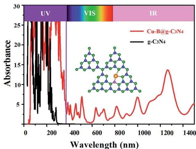
Fig. 5 Calculated optical adsorption spectrum for Cu–B atom pair decorated g-C<sub>3</sub>N<sub>4</sub> and pristine g-C<sub>3</sub>N<sub>4</sub>. The insert shows again the structure of the Cu–B@g-C<sub>3</sub>N<sub>4</sub> catalyst.
