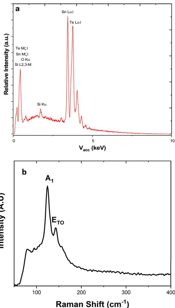
**Fig. 3** (a) EDX spectrum highlighting the elements present within the SnTe film, the silicon present is attributed to the substrate. (b) Raman spectrum with the data highlighting the A<sub>1</sub> and E modes at 124 and 143 cm<sup>-1</sup>, respectively.<sup>1</sup>
