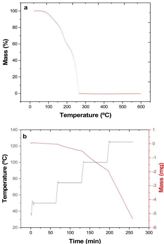
Fig. 1 (a) Thermogravimetric analysis of [<sup>n</sup>Bu<sub>3</sub>Sn(Te<sup>n</sup>Bu)] showing the percentage mass loss with temperature at a ramp rate of 5 °C min<sup>-1</sup> and a constant flow of argon gas. (b) Isothermal step TGA experiment of [<sup>n</sup>Bu<sub>3</sub>Sn(Te<sup>n</sup>Bu)] used for vapour pressure determination.
