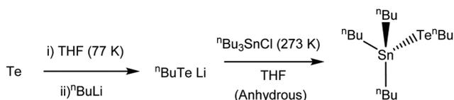
Scheme 1 Synthesis route to [<sup>n</sup>Bu<sub>3</sub>Sn(Te<sup>n</sup>Bu)].
