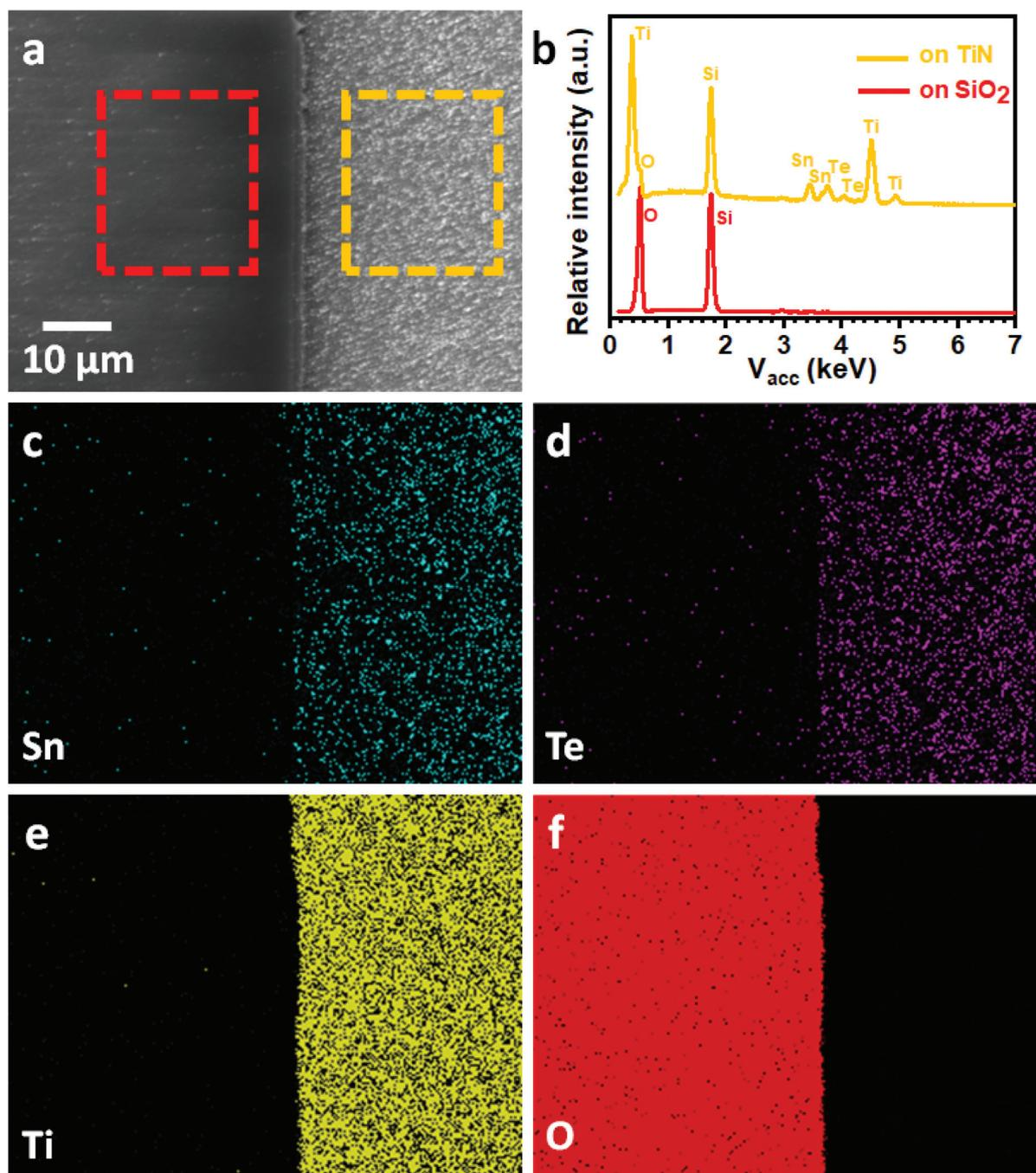
Fig. 5 (a) Top-view SEM image of a TiN/SiO<sub>2</sub> patterned substrate with SnTe selectively deposited on the TiN surface (right). (b) EDX spectra taken from the rectangular areas indicated in (a). EDX element mapping of (c) Sn, (d) Te, (e) Ti and (f) O.
