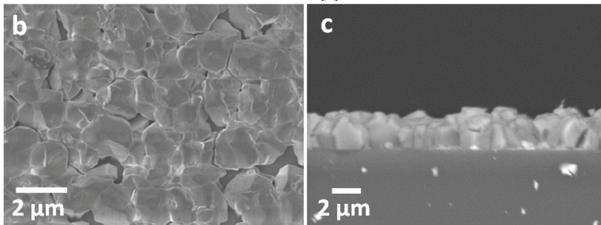
**Fig. 2** (a) Grazing incidence XRD pattern for SnTe thin film (thickness  $\sim 2 \mu\text{m}$ ) with XRD pattern for bulk cubic SnTe ( $Fm\bar{3}m$ ) (red).<sup>8</sup> The broad feature observed around  $21^\circ$  is due to the fused silica substrate beneath the SnTe film. Top down SEM (b) and cross-sectional SEM (c) of a SnTe film.
