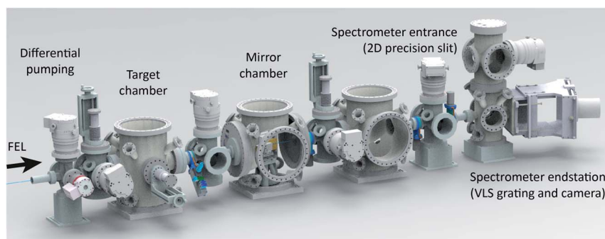
Fig. 2 Overview of the experimental vacuum apparatus. The FEL beam (coming from the left) is focused into the first large chamber (target chamber) downstream of a short differential pumping section. The second large chamber (mirror chamber) includes a toroidal mirror for refocusing into the spectrometer, and a two-component plane mirror for beam steering. The spectrometer endstation comprises a two-dimensional (two pairs of blades in the X- and Y-dimensions) motorized entrance slit, a highly-flexible assembly for many different beam attenuators, a variable-line-spacing (VLS) grating, and an XUV-sensitive camera (also see Fig. 3 and 4 for more details).
