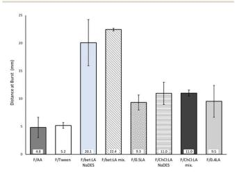
Fig. 2 Distance at burst (b) results of the different films.
