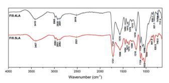
Fig. 5 FT-IR spectra of the F/0.4LA (black) and F/0.5LA (red).
