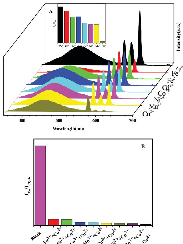
Fig. 5 (A) The emission spectra and the relative intensities of  $I_{613}/I_{450}$  for Eu-DPA-CQDs dispersed in different metal ion ( $10^{-3} \text{ mol L}^{-1}$ ) aqueous solutions. (B)  $I_{Eu}/I_{CQDs}$  of  $500 \text{ }\mu\text{M Cu}^{2+}$  ions and various co-existing metal ions.
