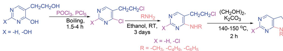
Scheme 19 Synthesis of 5,6-dihydropyrrolo[2,3- d ]pyrimidines.
