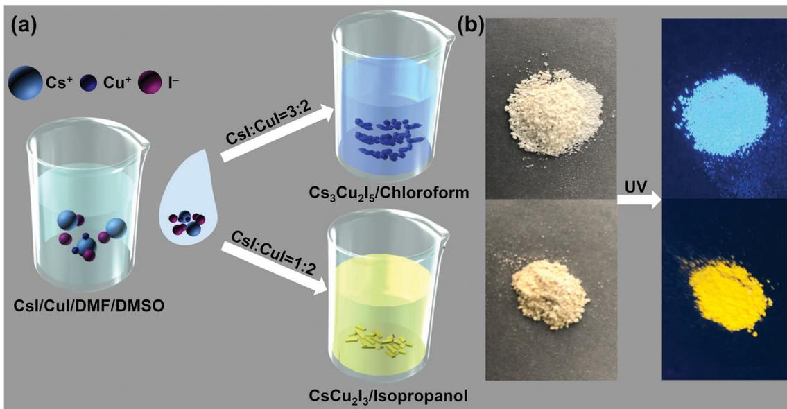
Fig. 1 (a) Schematic illustration of the reaction system for the supersaturated recrystallization technique at RT. (b) Photographs of synthesized  $\text{Cs}_3\text{Cu}_2\text{I}_5$  and  $\text{CsCu}_2\text{I}_3$  powders under sunlight (left) and 254 nm UV light irradiation (right).
