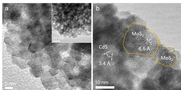
**Fig. 2** Representative (a) TEM and (b) HRTEM images of the 20-MoS<sub>2</sub>/CdS NCAs catalyst.
