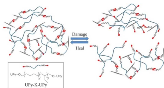
Fig. 6 Schematic of formation of supramolecular nanocomposites based on UPy-K-UPy and Upy-decorated CNCs. This figure has been adapted from ref. 41 with permission from American Chemical Society, copyright 2013.
