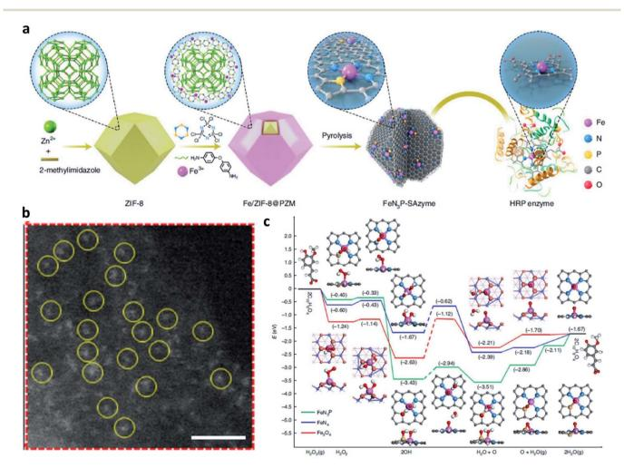
Fig. 11 (a) Schematic synthetic process of  $FeN_3P$ -SAzyme (SAzyme: single-atom nanozyme). (b) AC HAADF-STEM image of  $FeN_3P$ -SAzyme. Scar bar: 1 nm. (c) DFT calculations on the POD-like activity of  $FeN_3P$ -SAzyme,  $FeN_4$ -SAzyme, and  $Fe_3O_4$  nanozyme for comparison. Color code: C, grey; Fe, blue; N, light blue; O, light red; P, yellow; H, white. Reproduced with permission from ref. 57. Copyright 2021, Nature Publishing Group.
