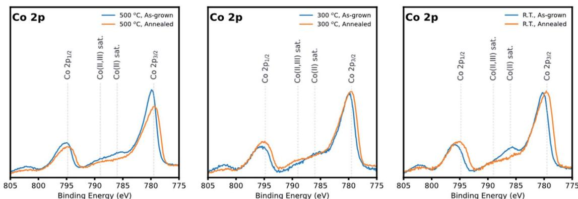
Fig. 5 X-ray photoelectron spectra of Co 2p of the LSC nanostructured films grown at  $500^\circ\text{C}$ ,  $300^\circ\text{C}$ , and R.T. As-grown films and annealed films are depicted in blue and orange, respectively.
