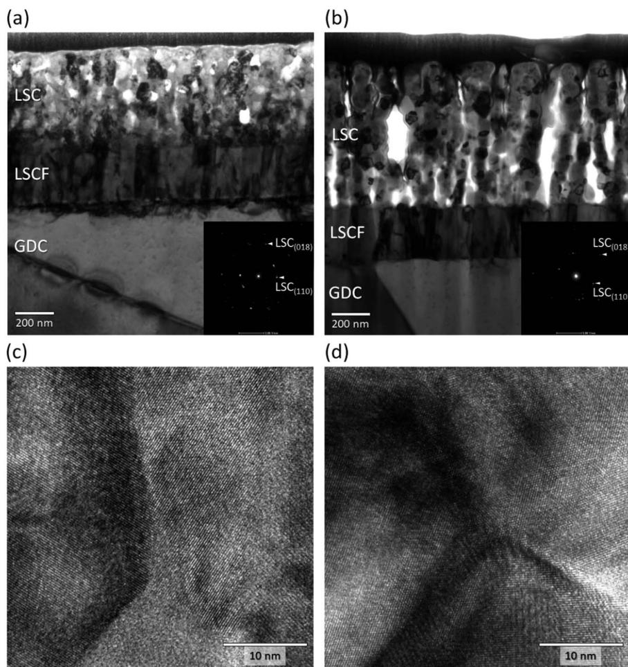
**Fig. 10** Representative TEM micrographs of LSC/LSCF/GDC symmetrical cells after long-term testing at 700 °C for 300 h in air. (a) LSC film prepared at 500 °C, (b) LSC film prepared at R.T. Insets are corresponding selected area electron diffraction patterns obtained in the respective LSC regions. High-magnification TEM micrographs showing lattice images taken near the surface of the (c) LSC film prepared at 500 °C, and (d) LSC film prepared at R.T.
