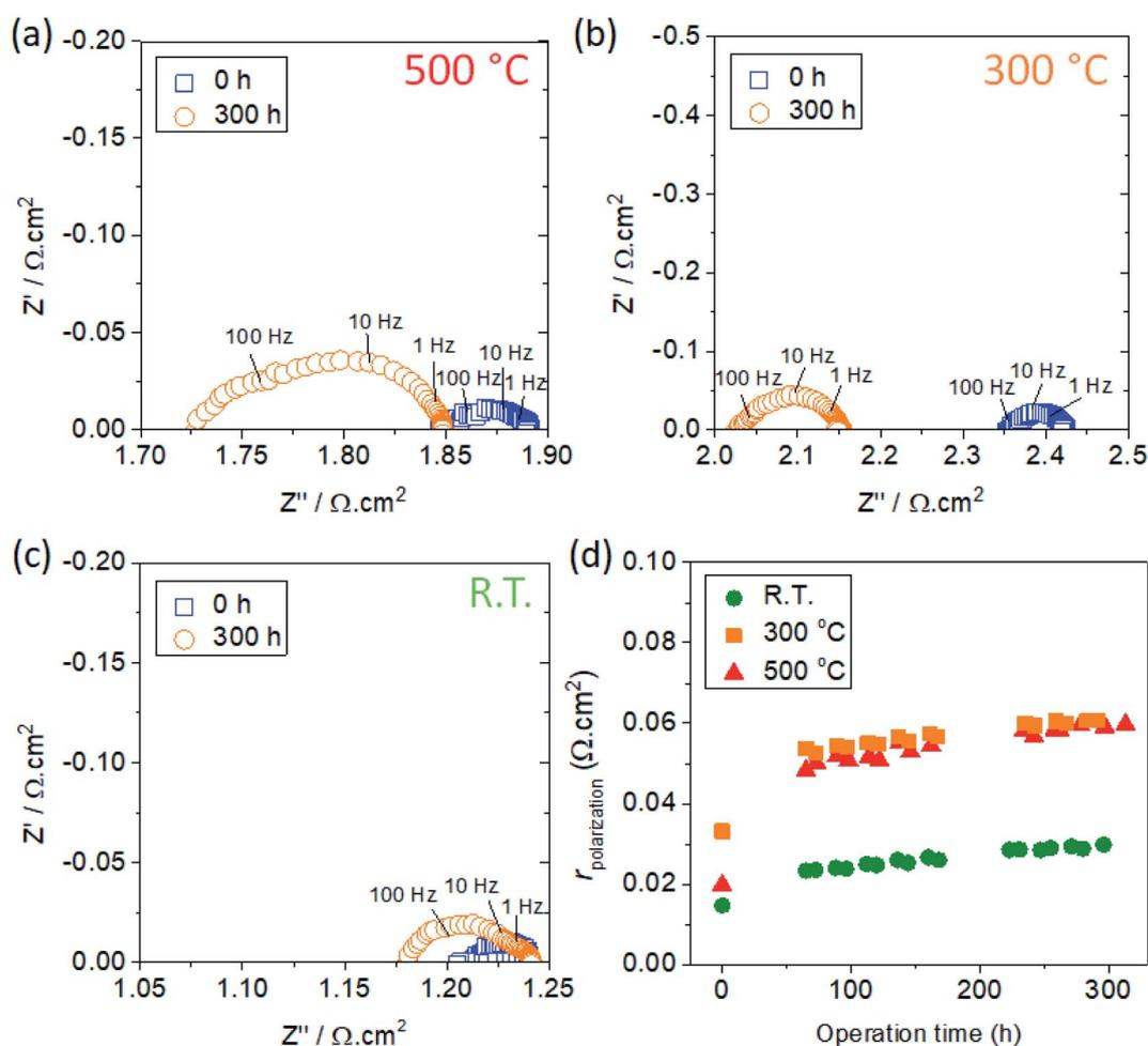
Fig. 8 Impedance spectra for LSC thin films deposited at (a) 500 °C, (b) 300 °C, and (c) room temperature (R.T.). The data at  $t = 0$  h and 300 h are depicted by square and circle symbols, respectively. The overall electrode resistance,  $r_{\text{polarization}}$ , is plotted versus operation time in (d). 500 °C: red triangles, 300 °C: orange squares, R.T.: green circles.
