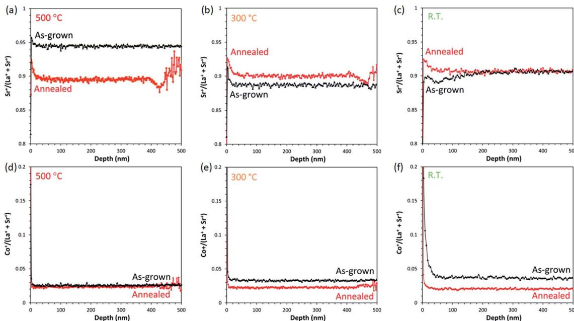
Fig. 6 Secondary ion ratios of  $\text{Sr}^+ / (\text{La}^+ + \text{Sr}^+)$  (top row) and  $\text{Co}^+ / (\text{La}^+ + \text{Sr}^+)$  (bottom row) derived from ToF-SIMS data for the as-grown and annealed LSC thin films prepared at 500 °C ((a) and (d)), 300 °C ((b) and (e)), and R.T. ((c) and (f)).
