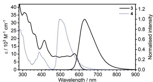
**Fig. 1** Comparison of absorption and photoluminescence spectra of complexes **3** and **4** in toluene,  $c = 10^{-5} \text{ M}$  for absorption and  $c = 5 \times 10^{-7} \text{ M}$  for emission spectra.
