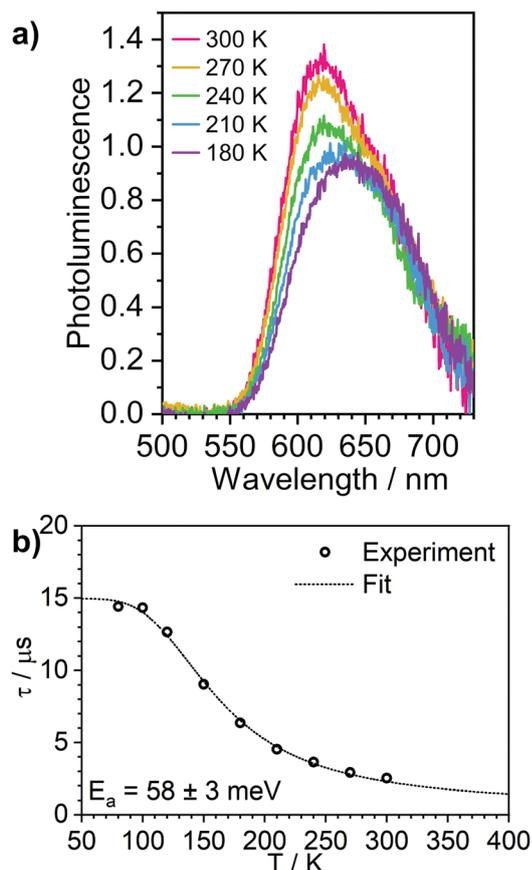
Fig. 6 Photoluminescence of **3** in polystyrene matrix at 0.1% (w/w). (a) steady state spectra recorded at temperatures from 300 to 180 K. (b) photoluminescence decay lifetime at temperatures from 300 to 80 K, showing the experimental data points and the best fit according to Eqn (1).
