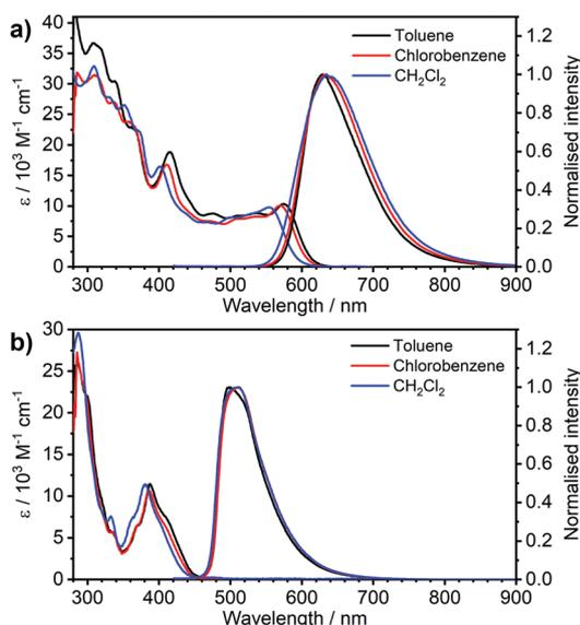
Fig. 2 Absorption and photoluminescence spectra of complexes (a) **3** and (b) **4** in the three solvents indicated in the figure legends,  $c \approx 10^{-5}$  M for absorption and  $c = 5 \times 10^{-7}$  M for emission spectra.
