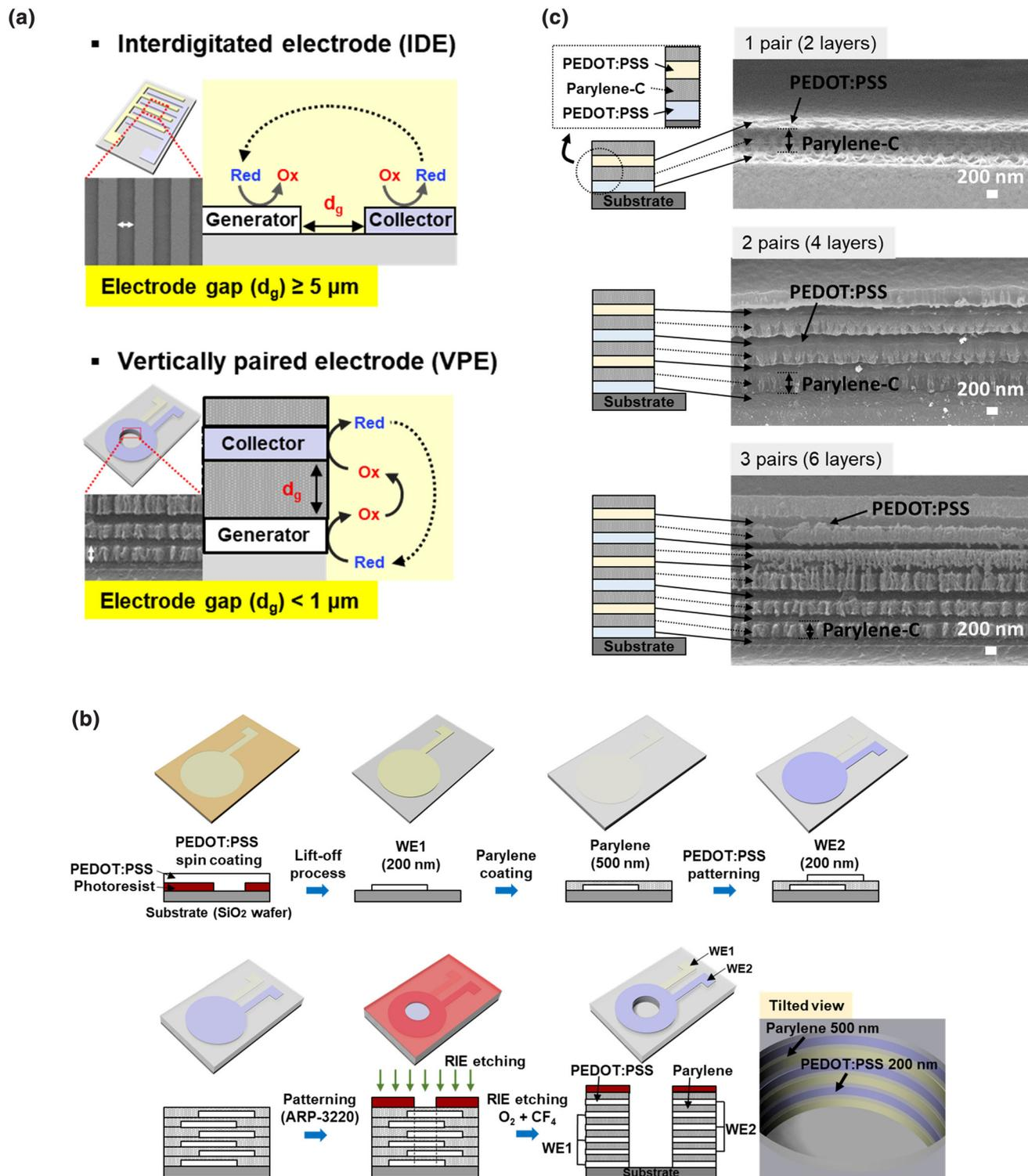
**Fig. 1** Fabrication procedure of the vertically paired electrode (VPE). (a) Comparison of an interdigitated electrode (IDE) and vertically paired electrode (VPE). (b) Fabrication process of the vertically paired electrode. (c) SEM images of VPEs with different numbers of electrodes.
