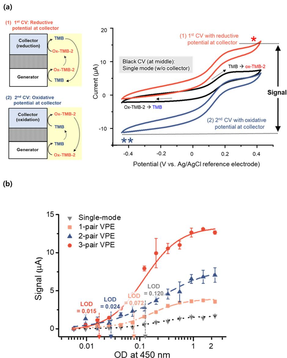
**Fig. 3** Redox cycling of TMB using the vertically paired electrode (VPE). (a) Redox cycling of TMB using the alternating potential of the collector electrode. (b) Standard curve for the redox cycling of ox-TMB-2 at different pairs of electrodes. (c) Comparison of the simulation and experimental data of the redox cycling signal for different electrode gaps. (d) Comparison of the simulated and experimental data of the redox cycling signal for different electrode pairs.
