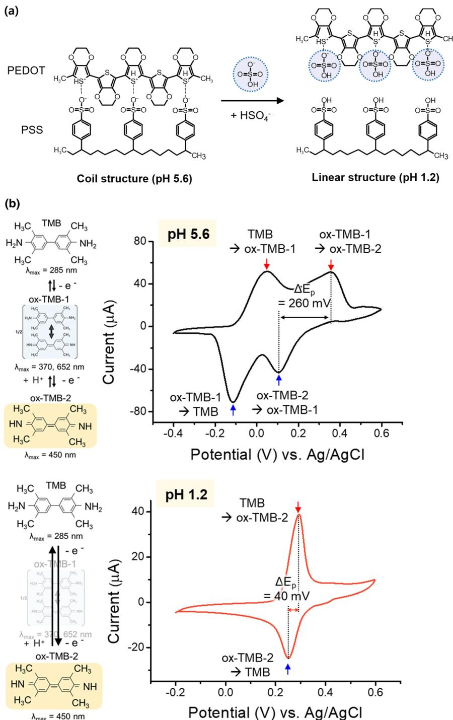
**Fig. 2** Electrochemical properties of PEDOT:PSS. (a) Structure of PEDOT:PSS at different pH values. (b) CV analysis of TMB at different pH conditions using the PEDOT:PSS electrode. (c) Conductivity and apparent electron transfer rate of PEDOT:PSS at different pH conditions. Inset presents the cyclic voltammogram of 50 mM ferricyanide + 1 M KCl for  $k_{\text{app}}$  estimation. (d) Double-layer capacitance of the PEDOT:PSS electrode at different pH conditions.
