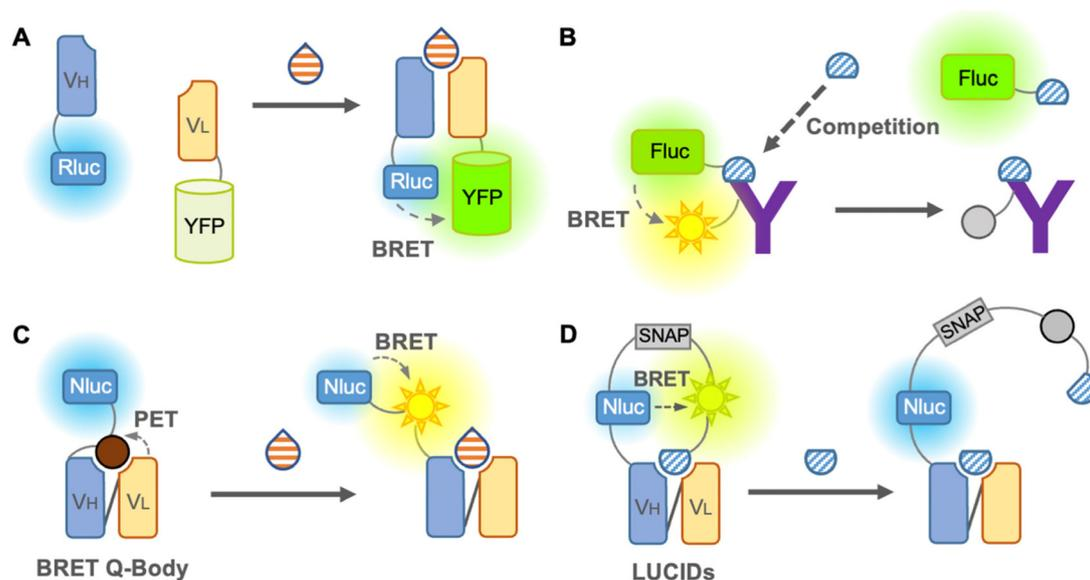
**Fig. 4** BRET immunosensors. (A) Scheme of an open sandwich BRET immunosensor. (B) Scheme of a competitive BRET immunosensor. (C) Scheme of a BRET-Q-body. (D) Scheme of a LUCID immunosensor. "Y" shape: antibody; semicircle: small molecule antigen; drop shape: large or small molecule antigen; and sun shape: fluorophore.
