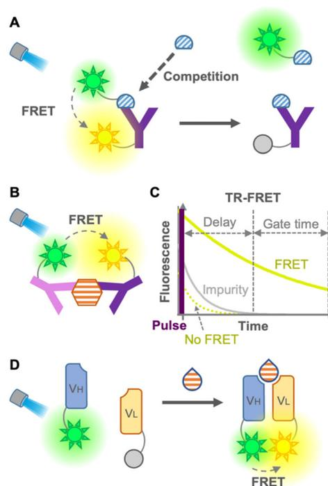
**Fig. 2** FRET immunosensors. (A) Scheme of a competitive FRET immunoassay. (B) Scheme of a non-competitive FRET immunoassay. (C) Principle of the TR-FRET immunoassay. Fluorescence from the acceptor (green) and impurity (gray). (D) Scheme of an open sandwich non-competitive immunoassay. "Y" shape: antibody; semicircle: small molecule antigen; hexagon: large molecule antigen; drop shape: large or small molecule antigen; and sun shape: fluorophore.
