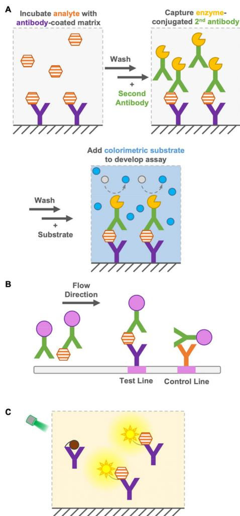
**Fig. 1** Heterogeneous and homogeneous immunoassays. (A) Scheme of a sandwich ELISA heterogeneous immunoassay with multiple incubation and washing steps. (B) Scheme of immunochromatography assay. (C) Example of a homogeneous immunoassay. "Y" shape: antibody; hexagon: antigen; gray or blue circle: colorimetric substrate or product; pink circle: colloidal gold; and sun shape: fluorophore.
