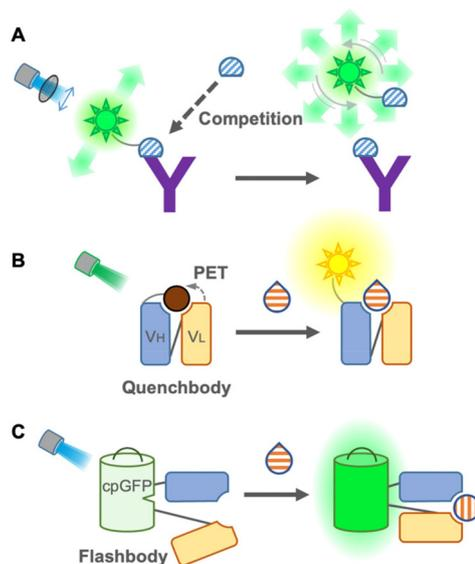
**Fig. 3** Single fluorophore immunosensors. (A) Scheme of a polarization-based immunosensor. (B) Scheme of a Quench-body (Q-body) immunosensor. (C) Scheme of a Flashbody immunosensor. “Y” shape: antibody; semicircle: small molecule antigen; drop shape: large or small molecule antigen; and sun shape: fluorophore.
