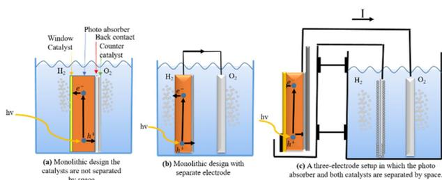
**Fig. 17** (a) Monolithic design where the catalysts are not separated by space. (b) Monolithic design with separated electrode. (c) A three-electrode setup in which the photoabsorber and both catalysts are separated by space.
