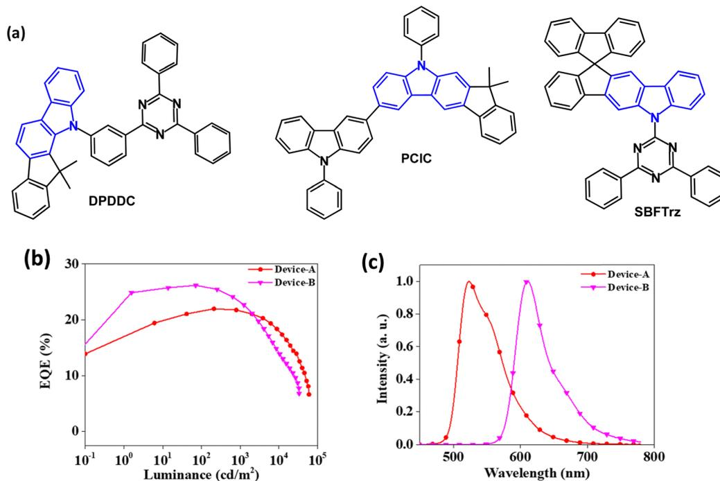
Fig. 6 (a) Molecular structures of indenocarbazoles **DPDDC**, **PCIC** and **SBFTzr**. (b) EQE-L data for **SBFTzr-Ir(ppy)<sub>2</sub>acac** (Device-A) and **SBFTzr-Ir(mphmq)<sub>2</sub>tmd** (Device-B).<sup>76</sup> (c) EL spectra of Device-A and Device-B.<sup>76</sup> Copyright 2021 Elsevier.
