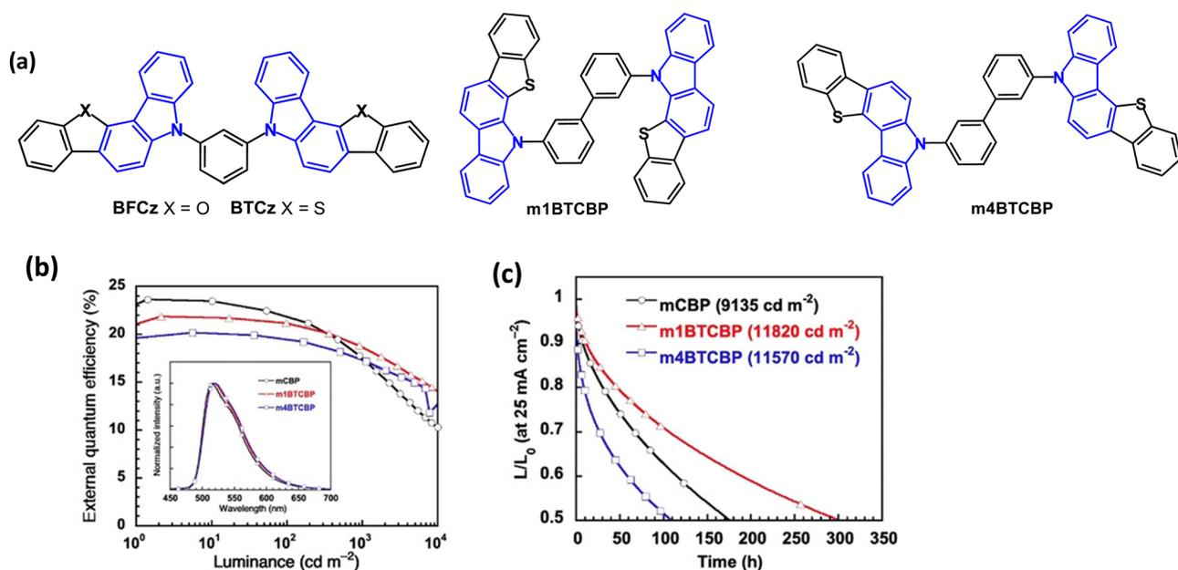
Fig. 8 (a) Molecular structures of **BFCz**, **BTCz**, **m1BTCBP** and **m4BTCBP**. (b) EQE–*L* characteristics.<sup>79</sup> (c) Operational lifetime at LT<sub>50</sub> with Ir(ppy)<sub>3</sub> emitter.<sup>79</sup> Copyright 2021 Wiley-VCH.
