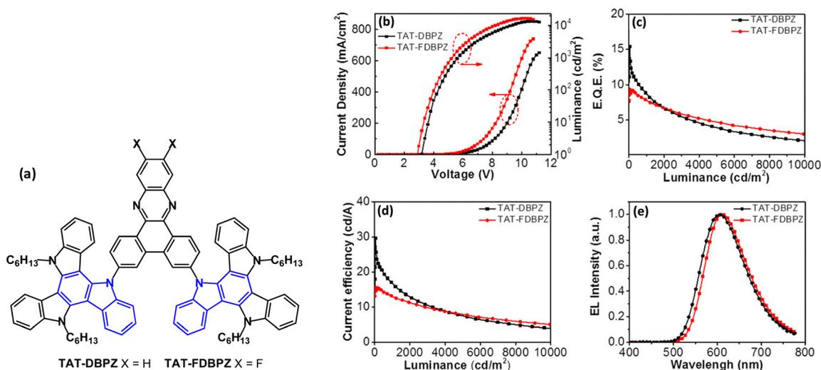
Fig. 26 (a) Molecular structures of **TAT-DBPZ** and **TAT-FDBPZ**. (b) Current density–voltage–luminance characteristics. (c) EQE–L curves. (d) CE–L curves. (e) EL spectra at 1000 cd m<sup>-2</sup>.<sup>144</sup> Copyright 2020 The American Chemical Society.
