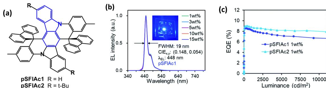
Fig. 45 (a) Molecular structures of pSFIac1 and pSFIac2. (b) EL spectra and (c) EQE–luminance curves.<sup>175</sup> Copyright 2022 The Royal Society of Chemistry.
