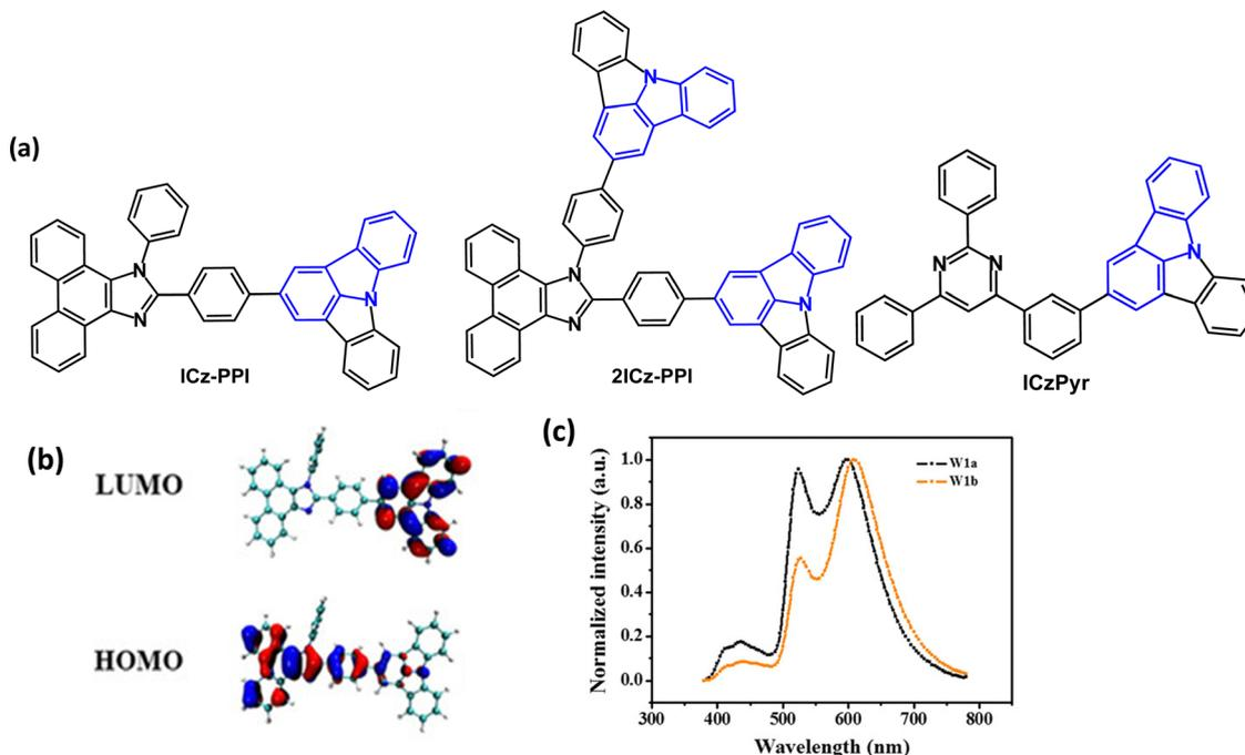
Fig. 7 (a) Molecular structures of **ICz-PPI**, **2ICz-PPI** and **ICzPyr**. (b) HOMO and LUMO plots for **ICz-PPI**.<sup>77</sup> (c) EL spectra of warm-white devices using  $\text{Ir}(\text{MDQ})_2(\text{acac})$ ,  $\text{Ir}(\text{ppy})_3$  and **ICz-PPI** in two different device configurations (W1a and W1b).<sup>77</sup> Copyright 2019 Wiley-VCH.
