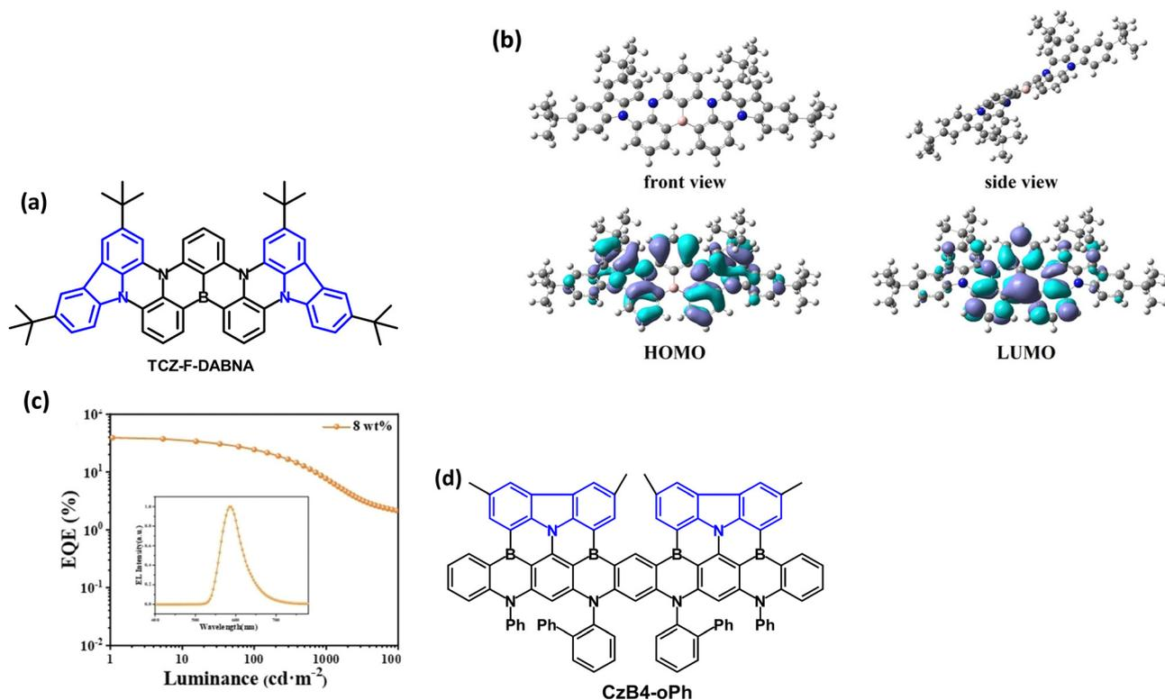
Fig. 38 (a) Molecular structure of **TCZ-F-DABNA**; (b) optimised molecular geometry and HOMO and LUMO distributions from DFT calculations; (c) EQE–L characteristics; inset shows the EL spectrum.<sup>162</sup> Copyright 2022 Wiley-VCH. (d) Molecular structure of **CzB4-oPh**.
