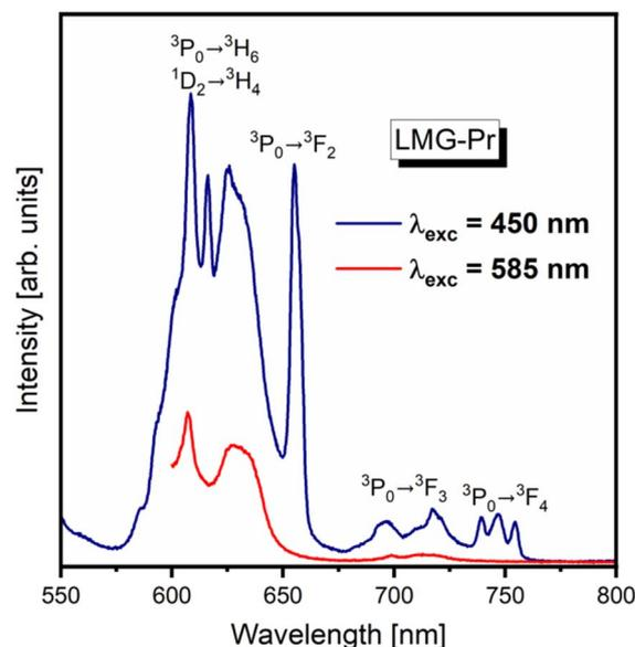
Fig. 8 Luminescence spectra of ceramic phosphors LMG-Pr excited at 450 nm ( $^3\text{P}_0$  state) and 585 nm ( $^1\text{D}_2$  state).
