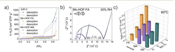
Fig. 3 Humidity-dependent proton conduction for Mn-HOFs, compared with JUK-2. (a) Water vapour adsorption at 293 K. (b) Representative temperature-dependent AC impedance plots for Mn-HOF-FA at 30% RH with equivalent circuit used for fitting. (c) Proton conductivities at 60 °C and different RH values (Mn-HOF-FA, Mn-HOF-MA and JUK-2 abbreviated FA, MA and AM, respectively).
