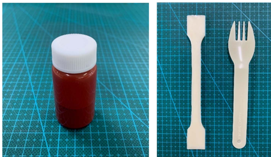
Fig. 35 Biomass biodegradable paint (Left) and plastic (Right) with anti-bacterial activity. 160
