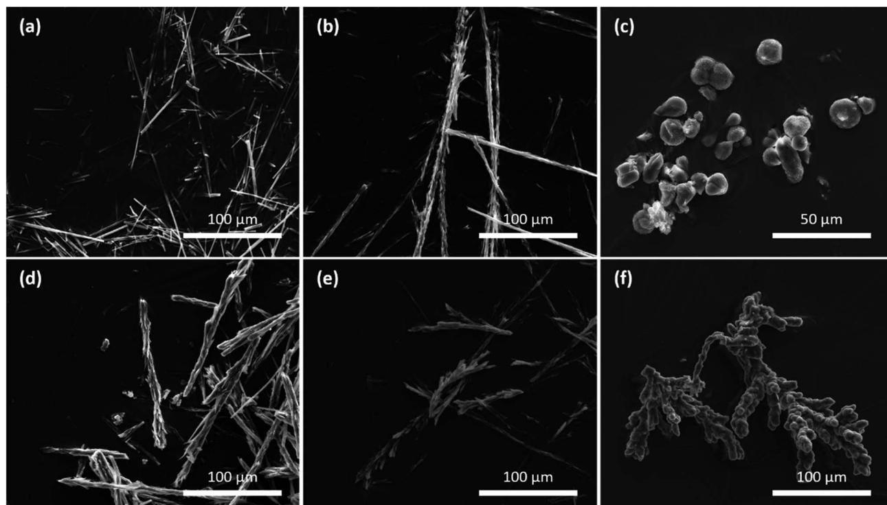
Fig. 4 SEM images of BSA@HOF composites showing crystals grown upon addition of  $\text{K}_2 \cdot 2$  at three different protein/total ligand ratios. Upon addition of *trans*- $\text{K}_2 \cdot 2$  at (a) 500 : 1; (b) 250 : 1; (c) 75 : 1; and *cis*- $\text{K}_2 \cdot 2$  at (d) 500 : 1; (e) 250 : 1; (f) 75 : 1.
