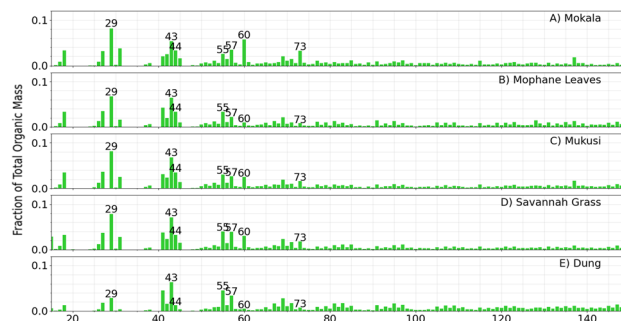
Fig. 2 Representative average OA mass spectra from the ACSM of controlled combustion experiments conducted without the introduction of humidity (RH < 10%) or external oxidants. Note data represents primary aerosol emissions from burning (A) mokala, (B) mopane leaves, (C) mukusi, (D) savannah grass, and (E) dung. ACSM measurements were taken within the first hour after combustion and is representative of data averaged over 15–20 min, which is 1 data point.
