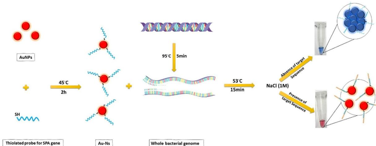
**Fig. 5** Colorimetric detection strategy for the *Staphylococcal* protein A (SPA) gene based on gold nanosensors (Au-Ns). AuNP surface is functionalized with a specific thiolated probe. *S. aureus* genome is denatured by heating at 95 °C for 5 min, then mixed with 50  $\mu$ L Au-Ns and incubated for 15 minutes. Finally, 5  $\mu$ L of NaCl solution was added to the mixture, and the result was evaluated by the naked eye.<sup>167</sup>
