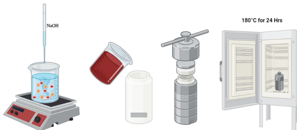
Scheme 1 Hydrothermal synthesis of the \text{CoFe}_2\text{O}_4/\text{Ni} foam electrodes.
