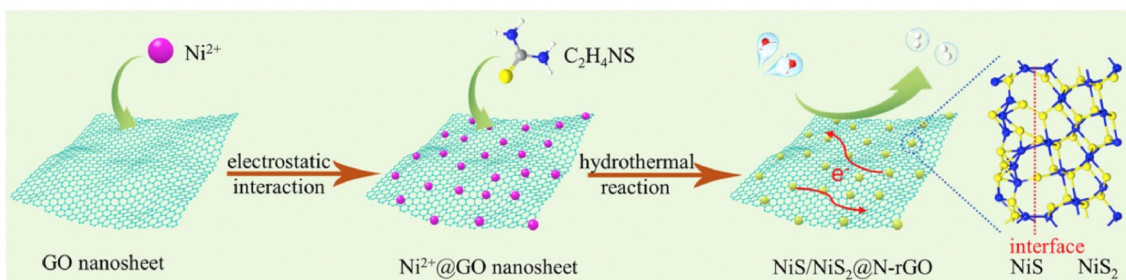
Fig. 5 Schematic reaction process for the synthesis of NiS/NiS 2 @N-rGO. Reprinted with permission from ref. 81. Copyright 2019, Elsevier.
