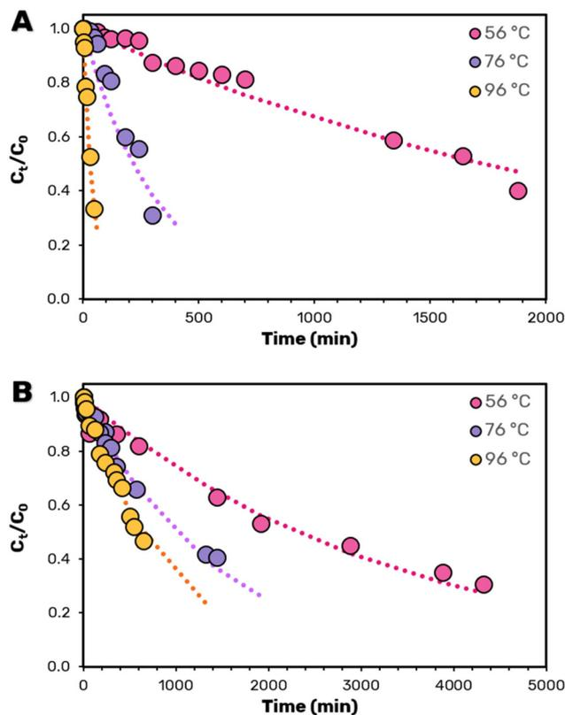
**Fig. 5** (A) Kinetic curves for carotenoid degradation as a function of temperature in the GVL extract (A) before and (B) after protein precipitation through the addition of ethanol. Dashed lines correspond to the polynomial order kinetic fitting using the  $k_d$  values listed in Table 2.
